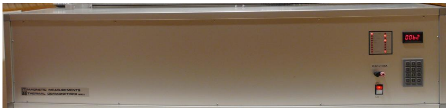
Figure 19 : Four à désaimantation MMTD18 (Magnetic Measurement).
