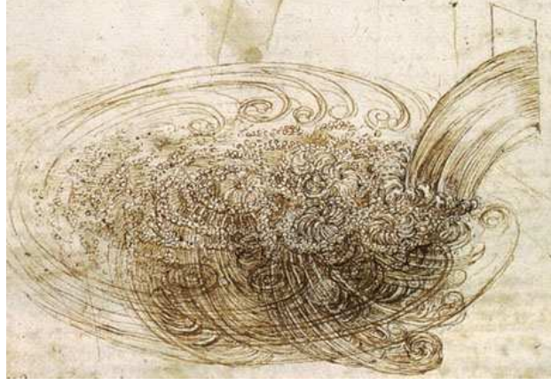
Figure 2.1: The first documented scientific study of turbulence is due to Leonardo Da Vinci in the sixteenth century. Here it is shown one of his drafts of a free water jet exiting from a square hole of a container into a pool.
