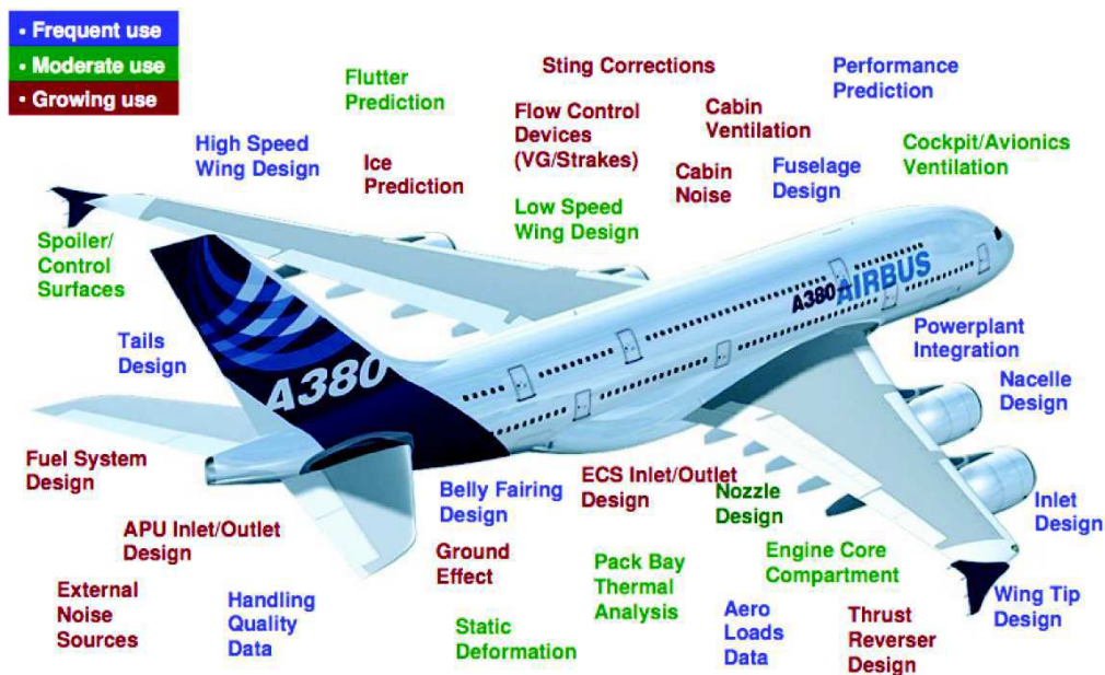
Figure 1.1: Use of CFD in aircraft development in Airbus [63].
