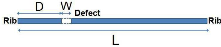
Figure 6.5: Geometry of defects in ribs.
