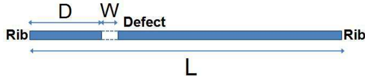
Figure 6.5: Geometry of defects in ribs.
