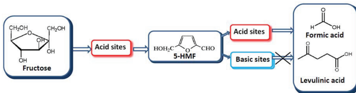
Scheme 5. 2. Influence of the acid-base properties on the product distribution in fructose dehydration in water.
