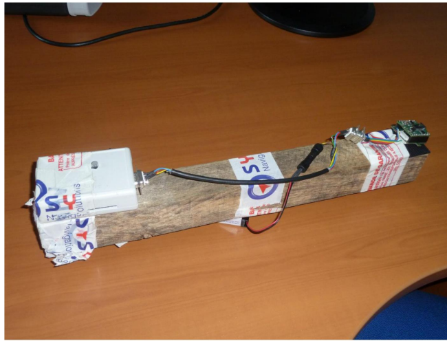
FIGURE 5.9: Image of three-axis magnetometer mounted on a wooden rod for calibration with the Earth magnetic field.
