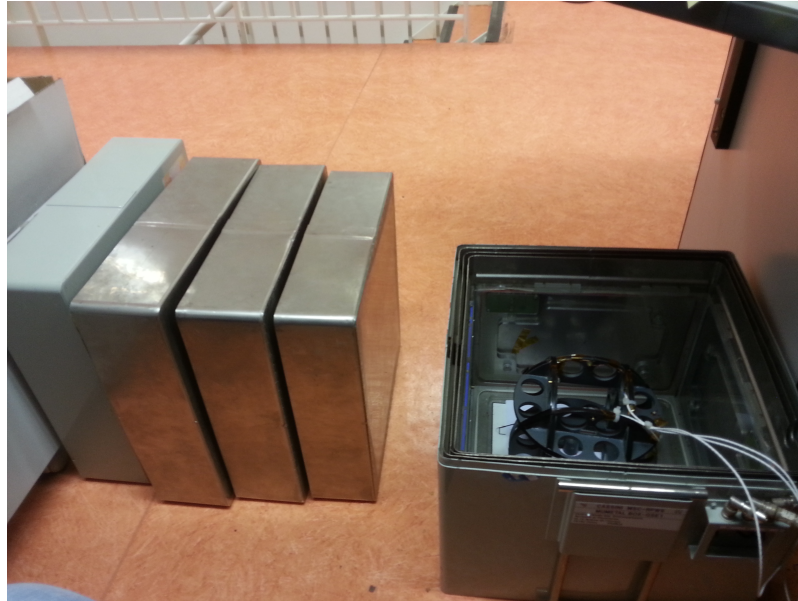
FIGURE 6.9: Photography of the mu-metal box.
