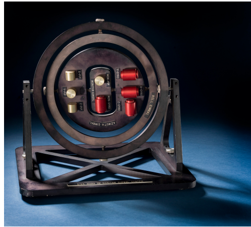
FIGURE 1.1: Model of Ship's Inertial Navigation stable platform made by Charles Stark Draper Laboratories.
