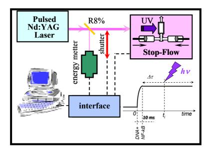
**Figure 7: Schematic representation of synchronized UV laser- stopped flow device:** The DNA and protein are injected by the syringes into the mixer and then into the quartz microcuvette where they are irradiated by a single UV laser pulse. The interface is a custom designed microprocessor controlled device that allows the synchronization of the UV laser and stopped flow device.
