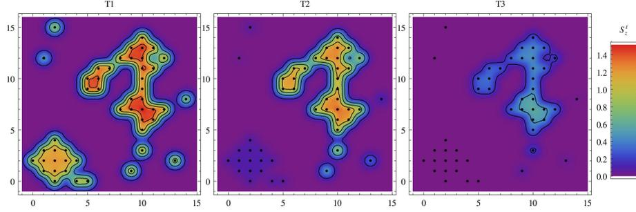
Figure 4.20: Snapshots of  $S_z^i$ 's corresponding to the case of  $x_{ns}=0.05$  for  $\lambda=a/2$ . From L-R:  $T_1$ ,  $T_2$ , and  $T_3$  denote the temperatures when  $\langle S_z^{avg} \rangle = 0.75S$ ,  $0.4S$  and  $0.1S$  respectively. (Here  $r_0=2a$ ,  $x_{in}=0.8$  and  $L=16$ ). (From Ref.[155]).
