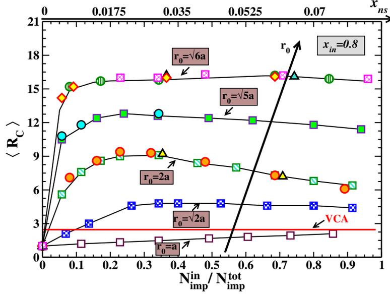
Figure 4.6:  $\langle R_C \rangle$  as a function of  $N_{imp}^{in}/N_{imp}^{tot}=(x_{in}/x)x_{ns}$  corresponding to  $\lambda=a/2$ . For a fixed  $x_{in}=0.8$  and different  $r_0$ . The upper  $x$ -axis represents the values of  $x_{ns}$  corresponding to  $x_{in}=0.8$ . The solid red line indicates the  $T_C^{VCA}$  scaled w.r.t  $\langle T_C^{hom} \rangle$ . (Here squares correspond to  $L=32$ , circles to  $L=36$ , triangles to  $L=40$  and diamonds to  $L=44$ ). (From Ref.[143]).
