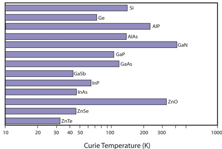
Figure 3.1: Predicted critical temperatures for different DMSs doped with 5% of Mn and containing  $3.5 \times 10^{20}$  holes/cm<sup>3</sup>. (From Dietl *et al.*[6]).
