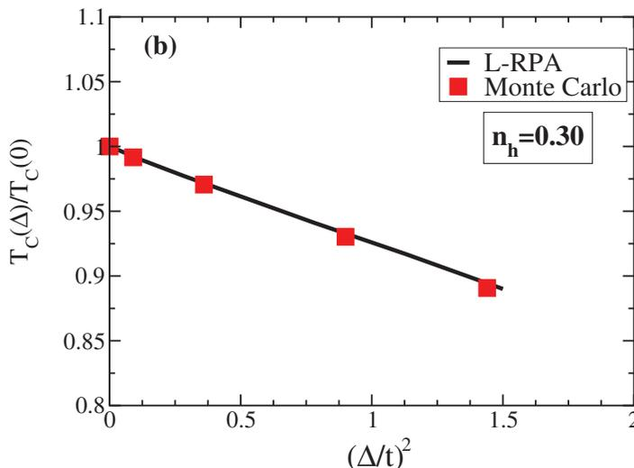
Figure 2.7:  $T_C$  for the double exchange model as a function of  $(\Delta/t)^2$  ( $\Delta$  is the on-site potential) for uncorrelated Anderson disorder. The solid line corresponds to the SC-LRPA and the squares represent values from MC simulations[64]. (From Ref.[60]).
