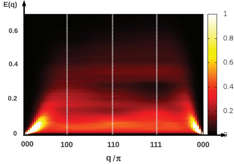
Figure 4.30: Spectral function  $A(\mathbf{q}, \omega)$  in the  $(\mathbf{q}, \omega)$  plane, corresponding to the homogeneous case for  $\lambda=a/2$ . The energy axis ( $y$ -axis) is in units of  $\omega/J_0$ . (Here  $N = 44^3$ ). (From Ref.[157]).
