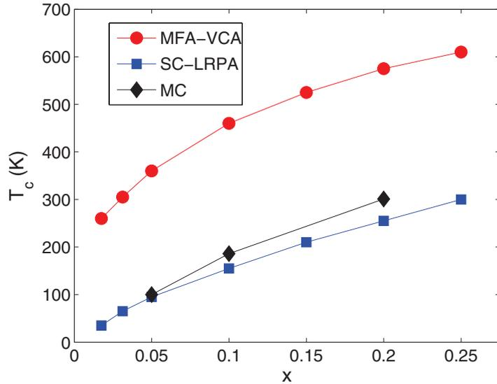
Figure 2.4: Curie temperatures of  $\text{Zn}_{1-x}\text{Cr}_x\text{Te}$  as a function of  $x$ , within the MFA-VCA, SC-LRPA, and MC simulations. (From Ref.[58]).
