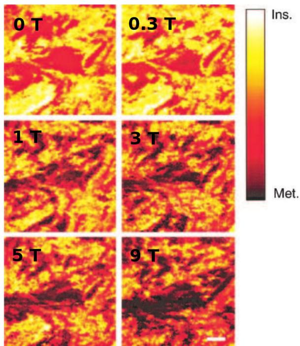
Figure 1.6: STS images of the local electronic structure of  $\text{La}_{0.7}\text{Ca}_{0.3}\text{MnO}_3$  taken just below  $T_C$  in magnetic fields from 0 to 9 T. Light (dark) colors correspond to the insulating (metallic) parts of the surface. (From Ref.[14]).
