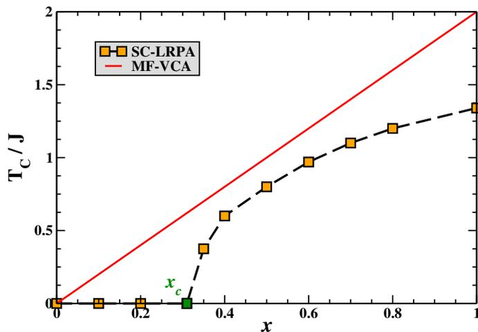
Figure 2.17: Curie temperature as a function of  $x$ . The solid (red) line is the MF-VCA  $T_C$  value. ( $x_c$  denotes the percolation threshold). (From Ref.[82]).
