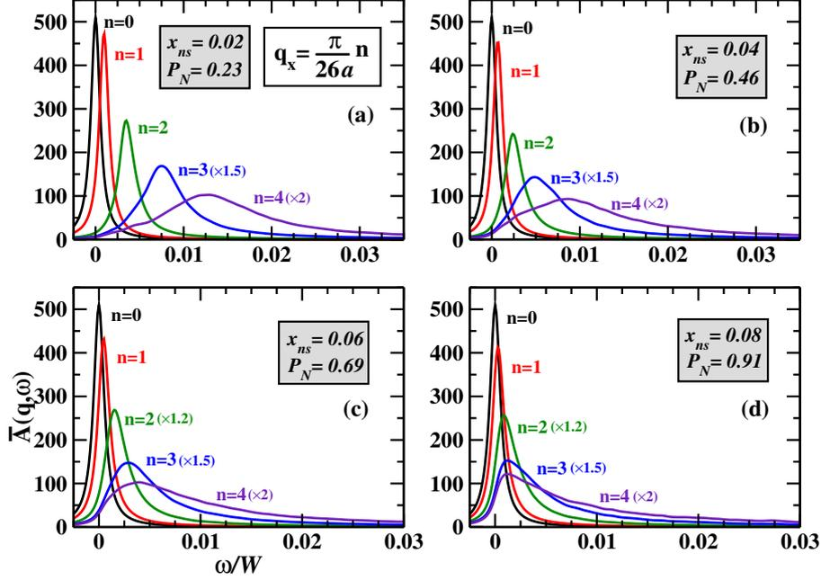
Figure 4.27: Average spectral function  $\bar{A}(\mathbf{q}, \omega)$  for the case of  $\lambda=a/2$ , with the other parameters same as in Figure 4.26. (From Ref.[156]).
