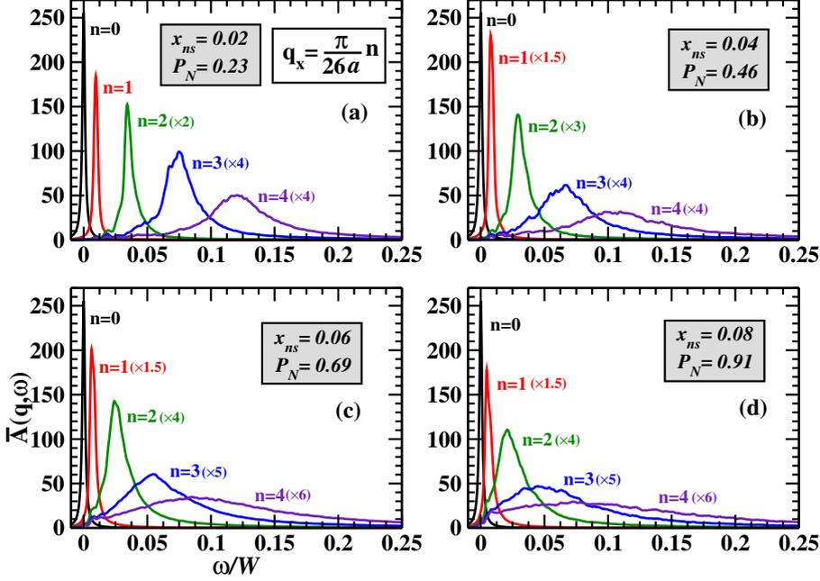
Figure 4.26: Average spectral function  $\bar{A}(\mathbf{q}, \omega)$  as a function of the energy in the (1 0 0) direction, for four different  $x_{ns}$ .  $P_N$  indicates the percentage of total impurities inside the nanospheres. The parameters are  $\lambda=a$ ,  $r_0=2a$ ,  $x_{in}=0.8$ , and  $N=52^3$ . The  $x$  axis is in units of  $\omega/W$ . (The intensity of the peaks have been multiplied by the factors indicated in the parentheses). (From Ref.[156]).
