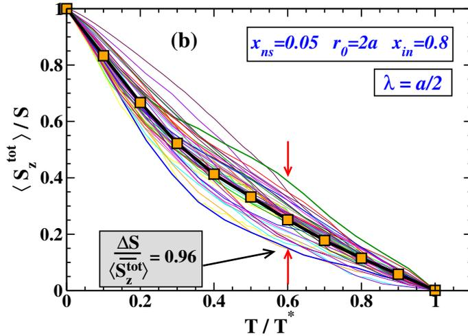
Figure 4.17: Total average magnetization as a function of  $T/T^*$  for  $x_{ns}=0.05$  calculated for 50 configurations (thin continuous lines), for  $\lambda=a/2$ . The thick black lines with symbols indicate the configuration averaged magnetization  $\langle S_z^{tot} \rangle$ .  $\frac{\Delta S}{\langle S_z^{tot} \rangle}$  is a measure of the fluctuation at  $T/T^*=0.6$ . (Here  $r_0=2a$ ,  $x_{in}=0.8$  and  $N=24^3$ ). (From Ref.[155]).
