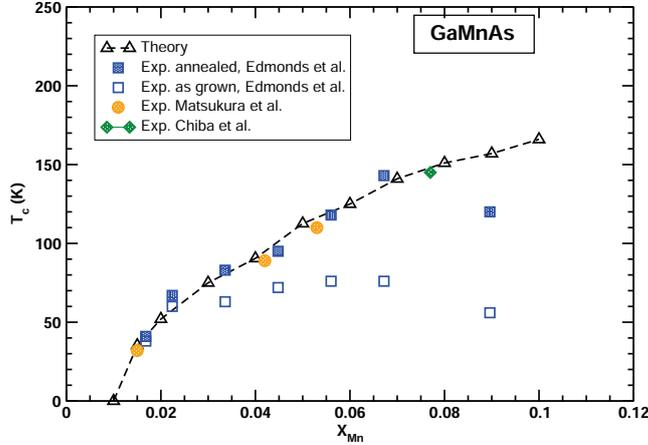
Figure 2.5: Curie temperature of  $\text{Ga}_{1-x}\text{Mn}_x\text{As}$  as a function of  $x$ . The triangles denote the calculated values within the SC-LRPA. The other symbols correspond to the experimental values. (From Ref.[57]).
