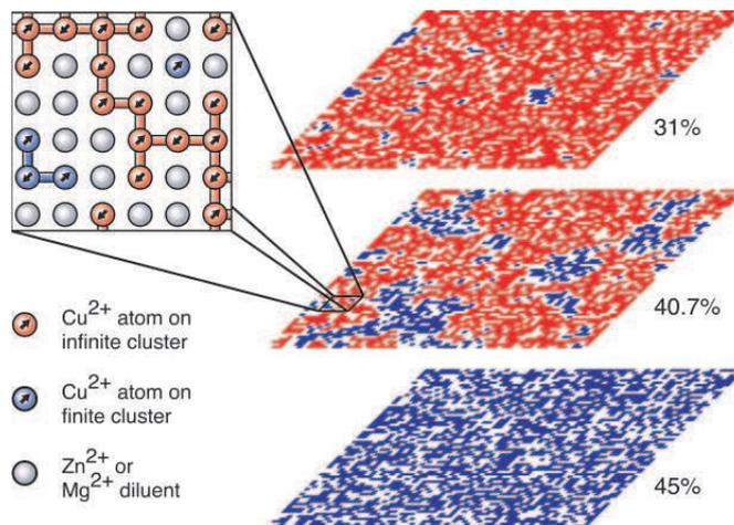
Figure 2.1: Schematic representation of finite-sized sections of an infinite square lattice for  $\text{La}_2\text{Cu}_{1-x}(\text{Zn},\text{Mg})_x\text{O}_4$ , for different site dilution levels. Inset: Close-up view for  $x=40.7\%$ , showing the role of magnetic Cu ions and non-magnetic Zn/Mg ions. (From Ref.[41]).
