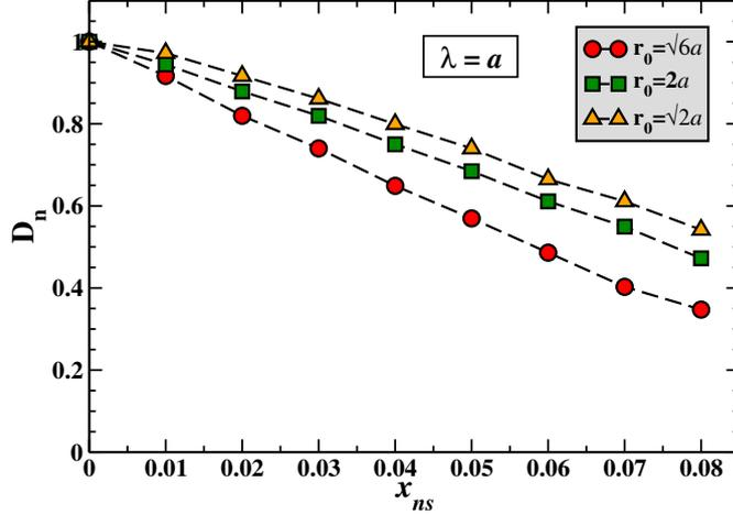
Figure 4.32: Normalized spin-stiffness  $D_n$  as a function of  $x_{ns}$ , for three different  $r_0$ :  $\sqrt{6}a$ ,  $2a$ , and  $\sqrt{2}a$ . (Here  $\lambda=a$  and  $x_{in}=0.8$ ). (From Ref.[156]).
