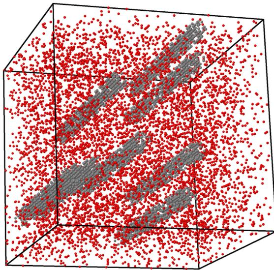
Figure 5.1: Snapshot of a simple cubic lattice containing nanocolumns. The grey (red) atoms denote the impurities inside (outside) the nanocolumns.
