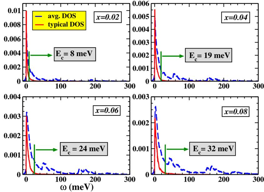
Figure 3.11: Magnon density of states as a function of the energy for four different  $x$ . The solid (dashed) lines represent the typical (average) density of states.  $E_c$  denotes the magnon mobility edge. (Here  $N = 44^3$ ). (From Ref.[111]).
