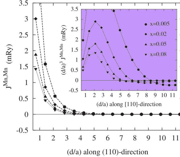
Figure 3.4: Exchange interactions in (Ga,Mn)As, along the (100) direction, for different Mn concentrations, as a function of the distance between the magnetic impurities. Inset: Same interactions scaled by a RKKY-like factor  $(d/a)^3$ . (From Ref.[92]).
