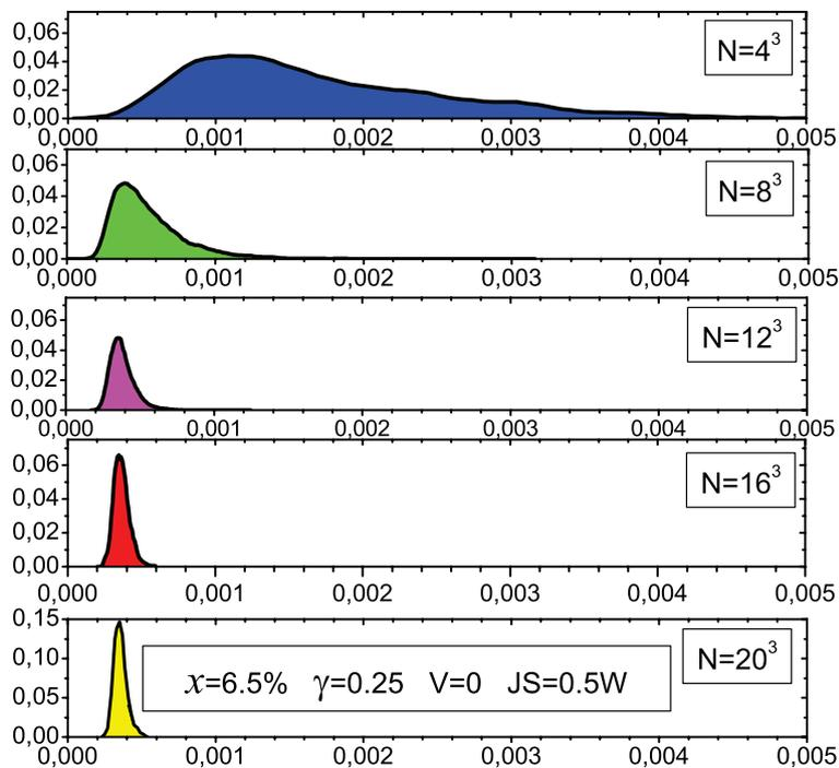
Figure 2.11: Distribution of the Curie temperatures (the x-axis is  $T_C$  in units of  $W$ ) for different system sizes  $N=L^3$ , where  $L$  varies from 4 to 20. The parameters are given in the figure. (From Ref.[66]).
