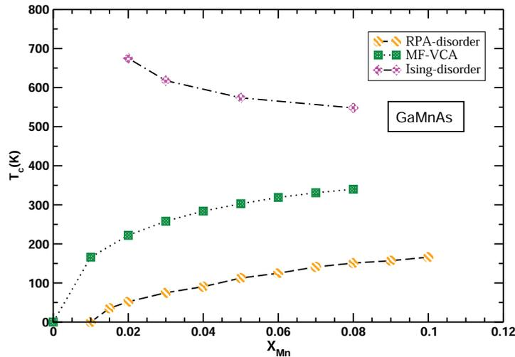
Figure 2.8: Curie temperature of (Ga,Mn)As as a function of  $x$ , for three different approximations , “Ising-disorder”, MF-VCA, and the SC-LRPA. (From Ref.[57]).
