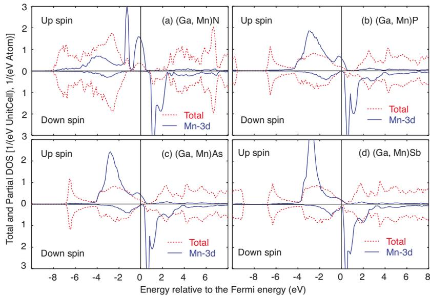
Figure 3.2: Density of states in (a)(Ga,Mn)N, (b)(Ga,Mn)P, (c)(Ga,Mn)As, and (d)(Ga,Mn)Sb. Total DOS (dotted lines) and partial density of 3d states (solid lines) at Mn site are shown. (From Ref.[53]).
