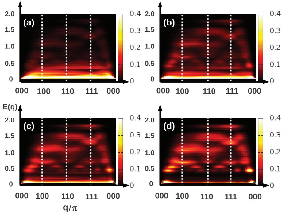
Figure 4.31: Spectral function  $A(\mathbf{q}, \omega)$  in the  $(\mathbf{q}, \omega)$  plane corresponding to  $\lambda=a/2$ , for four different  $x_{ns}$  : (a) 0.02, (b) 0.04, (c) 0.06, and (d) 0.08. The energy axis ( $y$ -axis) is in units of  $\omega/J_0$ . (Here  $r_0=2a$ ,  $x_{in}=0.8$ , and  $L=44$ ). (From Ref.[157]).
