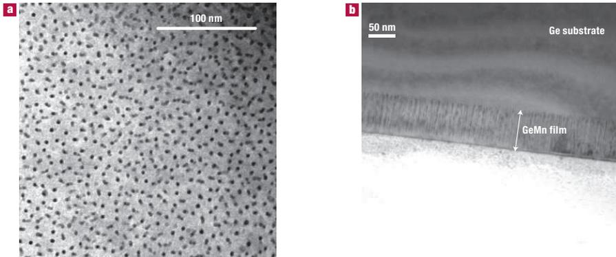
Figure 1.9: TEM images of a  $\text{Ge}_{0.94}\text{Mn}_{0.06}$  film. (a) Plane view where the dark spots are nanocolumns. (b) Cross-sectional view, where the nanocolumns are the dark lines which appear perpendicular to the film plane. (From Ref.[19]).
