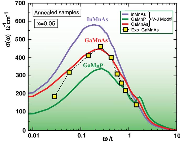
Figure 3.8: Optical conductivity as a function of  $\omega/t$  for optimally annealed (In,Mn)As, (Ga,Mn)As, and (Ga,Mn)P, for a Mn concentration of 5%. The symbols correspond to experimental data for (Ga,Mn)As. (From Ref.[97]).
