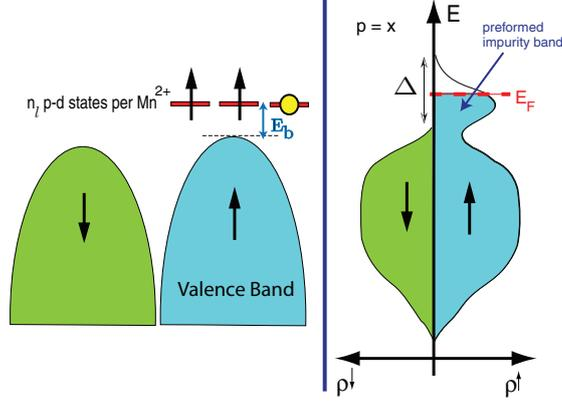
Figure 3.6: Left panel: Schematic representation of the 3  $p$ - $d$  states near the top of the valence band for (III,Mn)V compounds. Right panel: Spin resolved DOS and the formation of an impurity band for a finite Mn concentration (From Ref.[97]).
