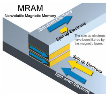
Figure 1.2: A schematic representation of magnetoresistive random-access memory (MRAM), which is based on the principle of GMR.
