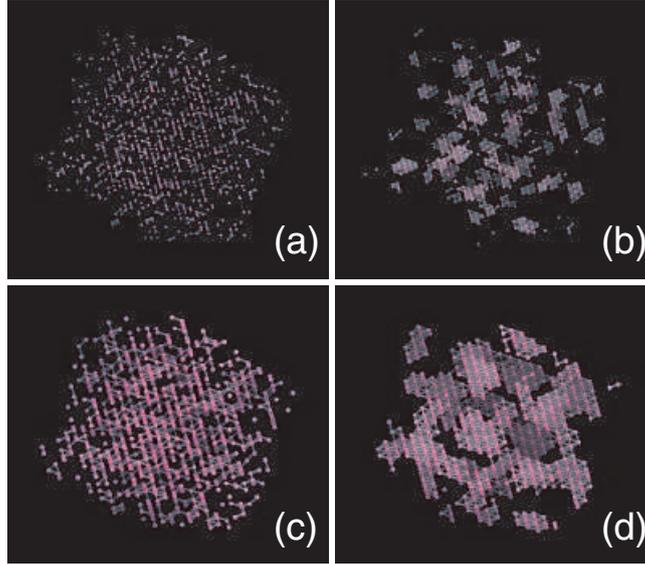
Figure 4.1: Snapshots (Ga,Mn)N for 5% Mn in (a) and (b), and 20% in (c) and (d). Random distributions in (a) and (c), and spinodal decomposition phases (after 100 MC steps) in (b) and (d). (From Ref.[134]).
