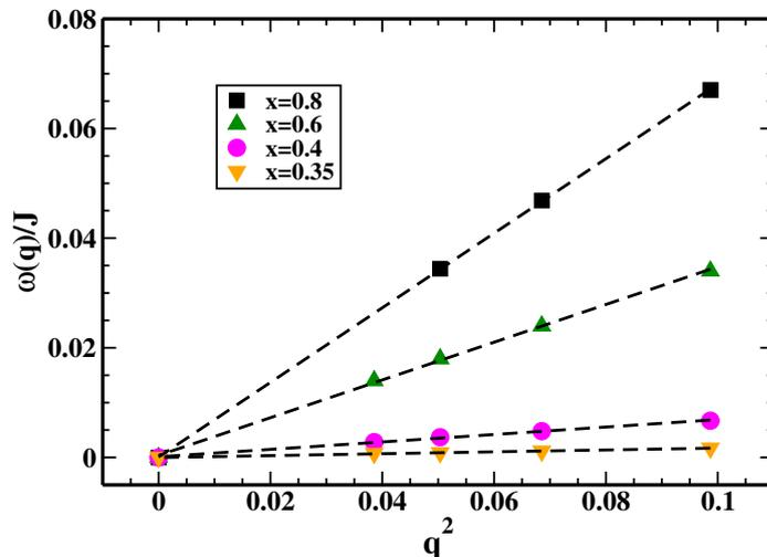
Figure 2.15: Magnon energy  $\omega(q)$  as a function of  $q^2$  for different values of  $x$ . Here  $L=20, 24, 28, \text{ and } 32$ . (From Ref.[72]).
