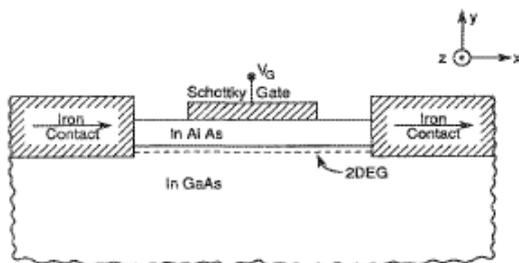
Figure 1.1: Original design of the SPINFET, as proposed by Datta and Das, from Ref. [1].
