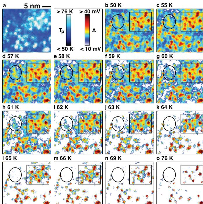
Figure 1.5: Evolution of the superconducting gap distribution with temperature in  $\text{Bi}_2\text{Sr}_2\text{CaCu}_2\text{O}_{8+\delta}$ . (a) Map of the local pairing temperature ( $T_p$ ). (b)–(o) A  $25 \times 28$  nm “gap-map” taken at different temperatures showing the distribution of gaps in real space. (From Ref.[13]).
