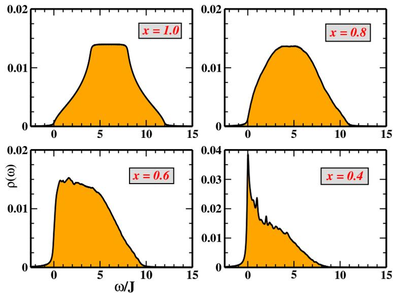
Figure 2.12: Magnon density of states  $\rho(\omega)$  as a function of the energy  $\omega$  for four different  $x$ . The energy axis (x-axis) is in units of  $\omega/J$ . (From Ref.[72]).
