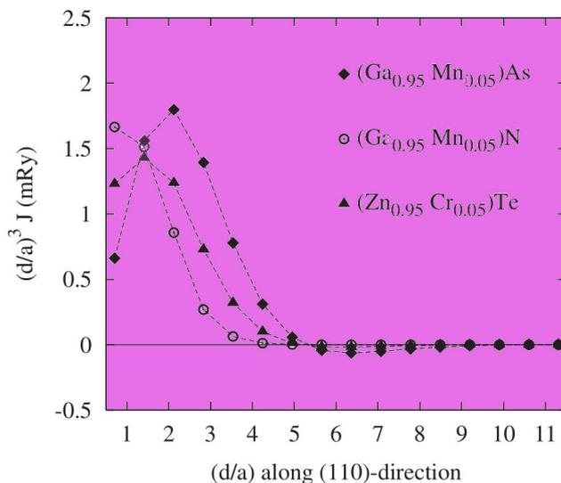
Figure 3.3: Mn-Mn exchange interactions, scaled by a RKKY-like factor  $(d/a)^3$ , in the (1 0 0) direction for (Ga,Mn)As, (Ga,Mn)N, and (Zn,Cr)Te. (From Ref.[92]).
