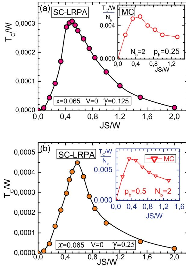
Figure 2.9: Curie temperature (in units of the bandwidth  $W$ ) within SC-LRPA as a function of  $JS/W$  for a fixed  $x=6.5\%$ . The hole concentration per impurity is (a)  $\gamma=0.125$ , and (b)  $\gamma=0.25$ . The insets show the MC results for a two-band model ( $N_b=2$ ) where the density of holes  $p_h=2\gamma$ . (From Ref.[66]).
