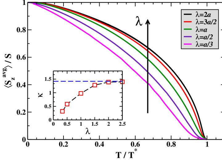
Figure 4.12: Average magnetization as a function of  $T/T^*$  for different values of  $\lambda$ , corresponding to the homogeneous case for one configuration. (Inset) Curvature of the  $\langle S_z^{avg} \rangle$  curves as a function of  $\lambda$ , calculated at  $T/T^*=0.5$ . (Here  $N=24^3$ ). (From Ref.[155]).
