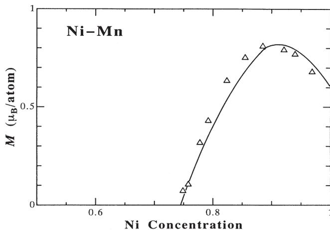
Figure 2.2: Magnetization of a Ni-Mn system, calculated within the KKR-CPA method, as a function of the Ni concentration. The triangles represent experimental data from Ref.[49]. (From Ref.[48]).
