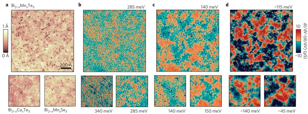
Figure 1.8: (a) STM images on the surface of Mn and Ca doped  $\text{Bi}_2\text{Te}_3$  and Mn doped  $\text{Bi}_2\text{Se}_3$ . (b)-(d) Conductance maps taken at high, intermediate and low sample biases. (From Ref.[17]).
