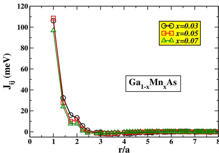
Figure 3.9: Exchange couplings in well annealed  $\text{Ga}_{1-x}\text{Mn}_x\text{As}$  as function of the distance between the impurities, for three different  $x$ . (From Ref.[111]).
