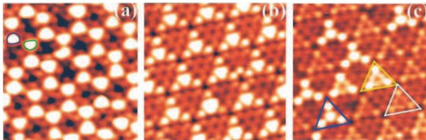
Figure 1.3: (a) Mixed array of equal-size In and Mn clusters, (b) Identical In/Ag alloy cluster array, and (c) STM image for the surface with low In/Ag coverage, demonstrating that the nanoclusters in (b) are In/Ag alloy. (From Ref.[11]).
