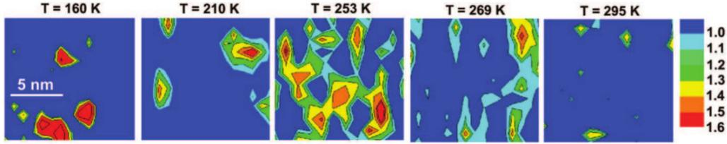
Figure 1.7: Intensity maps of the superlattice reflections in  $\text{La}_{0.55}\text{Ca}_{0.45}\text{MnO}_3$  at different temperatures moving across FM-PM phase transition. Each map is from an area of  $12 \times 12 \text{ nm}^2$ . (From Ref.[15]).
