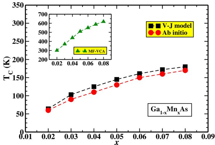
Figure 3.10: Curie temperature as a function of  $x$  in well annealed  $\text{Ga}_{1-x}\text{Mn}_x\text{As}$ . The squares (circles) represent the  $V$ - $J$  model (*ab initio*) calculations. Inset: MF-VCA  $T_C$  (in K) as a function of  $x$ . (From Ref.[111]).
