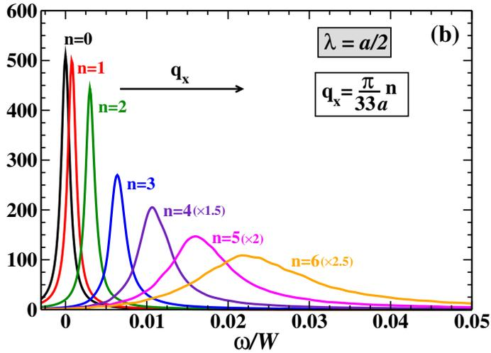
Figure 4.25: Average spectral function  $\bar{A}(\mathbf{q}, \omega)$  as a function of the energy in the (1 0 0) direction for different values of  $q_x$ , corresponding to the homogeneous case for  $\lambda = a/2$ . The energy axis ( $x$ -axis) is in units of  $\omega/W$ . The system size is  $N=66^3$ . (The intensity of the peaks have been multiplied by the factors indicated in the parentheses). (From Ref.[156]).
