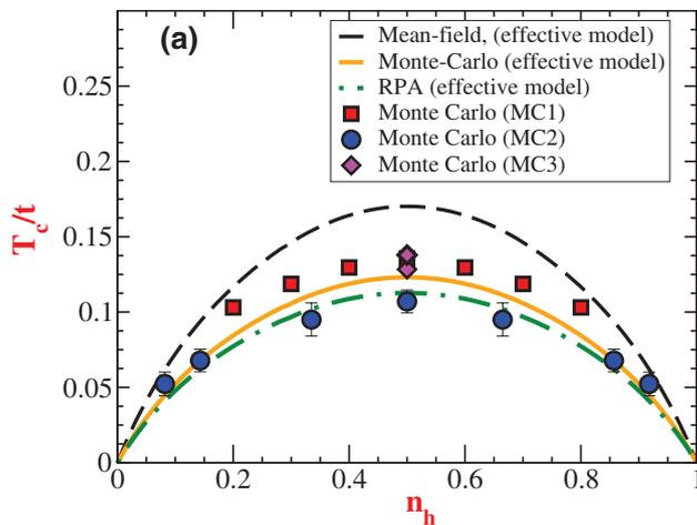
Figure 2.6:  $T_C$  for the double exchange model as a function of  $n_h$  corresponding to the clean case. The dashed, solid, and dot-dashed lines are obtained with the MF, MC, and RPA treatments, respectively. The symbols indicate the MC treatment of the full double exchange model. (From Ref.[60]).
