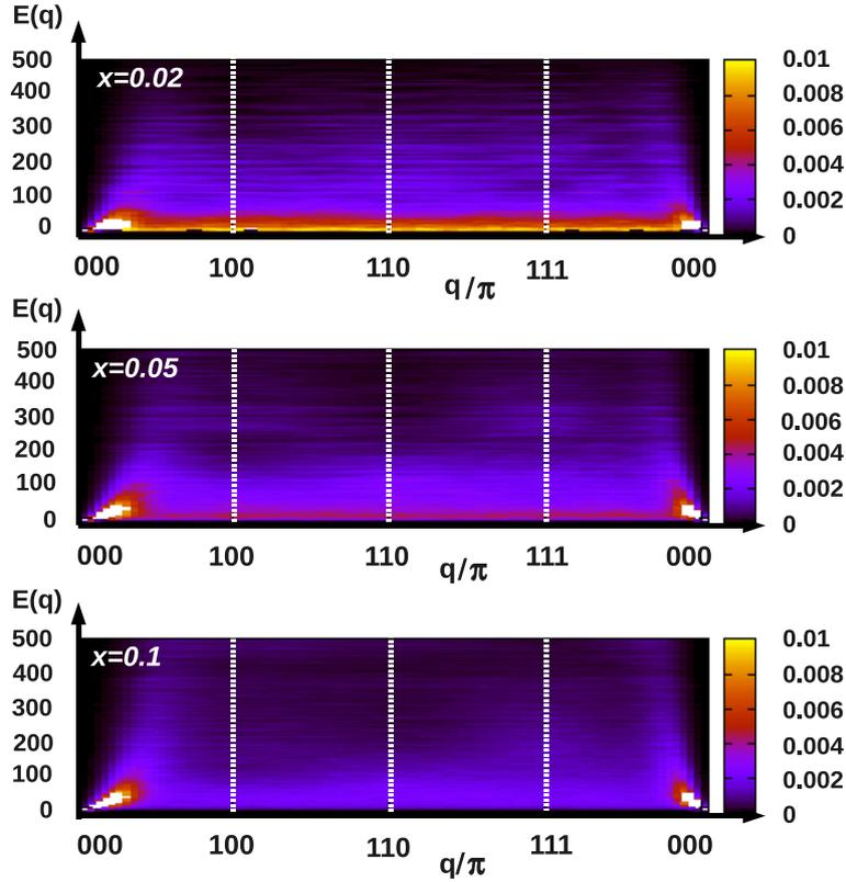
Figure 3.12: Spectral function  $A(\mathbf{q}, \omega)$  in the  $(\mathbf{q}, \omega)$  plane for three different Mn concentrations ( $x$ ). The energy axis ( $y$  axis) is in meV. (Here  $N = 44^3$ . (From Ref.[111]).
