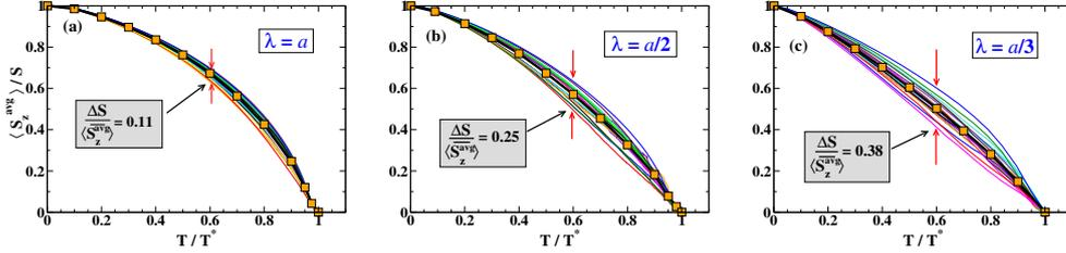
Figure 4.13: Average magnetization for the homogeneous case calculated for 25 configurations, for (a)  $\lambda=a$ , (b)  $\lambda=a/2$ , and (c)  $\lambda=a/3$ . The thick black lines with symbols indicate the configuration averaged magnetization.  $\frac{\Delta S}{\langle S_z^{avg} \rangle}$  is a measure of the fluctuation at  $T/T^*=0.6$ . (Here  $N=24^3$ ). (From Ref.[155]).
