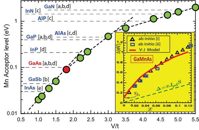
Figure 3.5: Mn acceptor level  $E_b$  (eV) as a function of  $V/t$  in III-V hosts (assuming  $t \approx 0.7$  eV and  $J_{pd}S = 4.3t$ ). Inset: Spin splitting  $\Delta$  as a function  $x$  in  $\text{Ga}_{1-x}\text{Mn}_x\text{As}$ . (From Ref.[97]).
