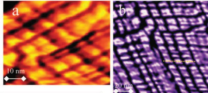
Figure 1.4: STM images on the surface of boron-doped diamond microcrystals. The image sizes are (a)  $620 \times 500 \text{ \AA}^2$ , and (b)  $1300 \times 1300 \text{ \AA}^2$ . (From Ref.[12]).
