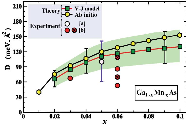
Figure 3.14: Spin-stiffness (in  $\text{meV}\cdot\text{\AA}^2$ ) as a function of  $x$ . Squares correspond to the  $V$ - $J$  model, hexagons to *ab initio* values[81] and circles [a,b] to experimental values from Ref.[119, 120]. The green shaded region corresponds to the errors bars for the  $V$ - $J$  model (see text for details). (Note the circles with a cross represent the annealed samples from Ref.[120]). (From Ref.[111]).
