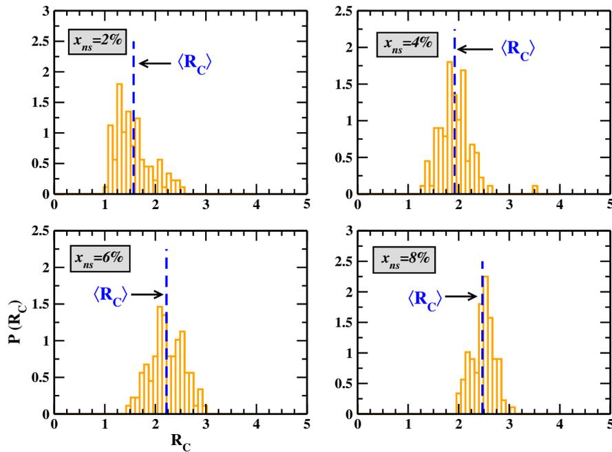
Figure 4.8: Normalized  $R_C$  distributions for four different  $x_{ns}$ : 0.02, 0.04, 0.06, and 0.08 corresponding to  $\lambda=a$ . Here  $r_0=2a$ ,  $x_{in}=0.8$  and  $L=32$ . The blue dashed lines indicate the  $\langle R_C \rangle$  values which we have shown in Figure 4.5. (From Ref.[144]).
