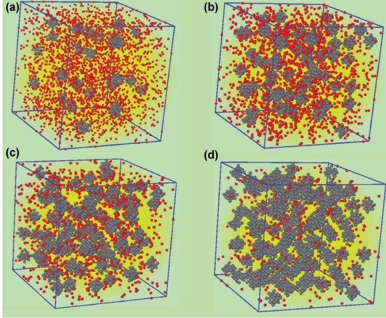
Figure 4.3: Snapshots corresponding to four different concentrations of nanospheres  $x_{ns}$  (a) 0.02, (b) 0.04, (c) 0.06 and (d) 0.08. The grey (red) atoms denote the impurities inside (outside) the nanospheres. (Here  $L=36$ ,  $r_0=2a$ , and  $x_{in}=0.8$ ). (From Ref.[143]).
