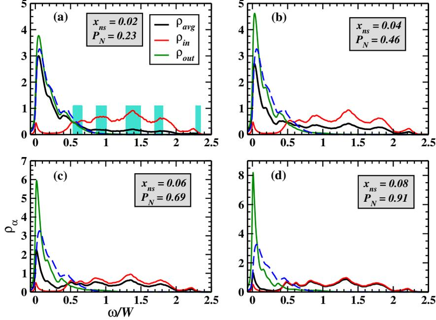
Figure 4.23:  $\rho_{avg}$ ,  $\rho_{in}$ , and  $\rho_{out}$  for  $\lambda=a/2$ , for four different  $x_{ns}$ . The shaded regions in (a) correspond to the calculated eigenmodes of a single isolated nanosphere. The other parameters being same as in Figure 4.22. The homogeneous magnon bandwidth is  $W \approx 0.8J_0$ . The blue dashed curve indicates the homogeneous  $\rho_{avg}$  from Figure 4.21(b). (From Ref.[156]).
