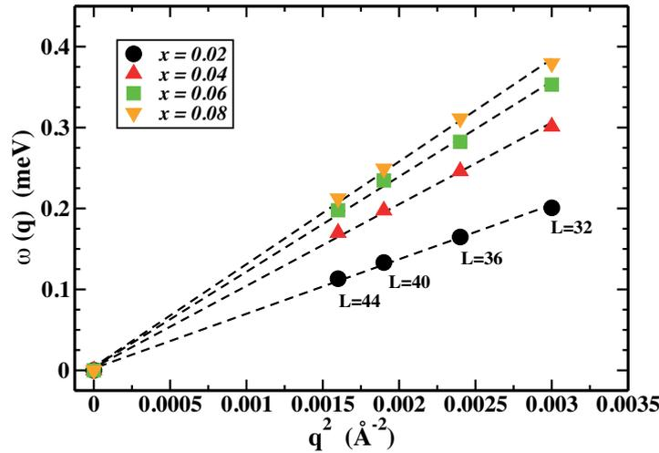
Figure 3.13: Magnon energy  $\omega(\mathbf{q})$  as a function of  $\mathbf{q}^2$  for different concentrations of Mn ( $x$ ). ( $N=L^3$ , where  $L=32, 36, 40$ , and  $44$ ). (From Ref.[111]).
