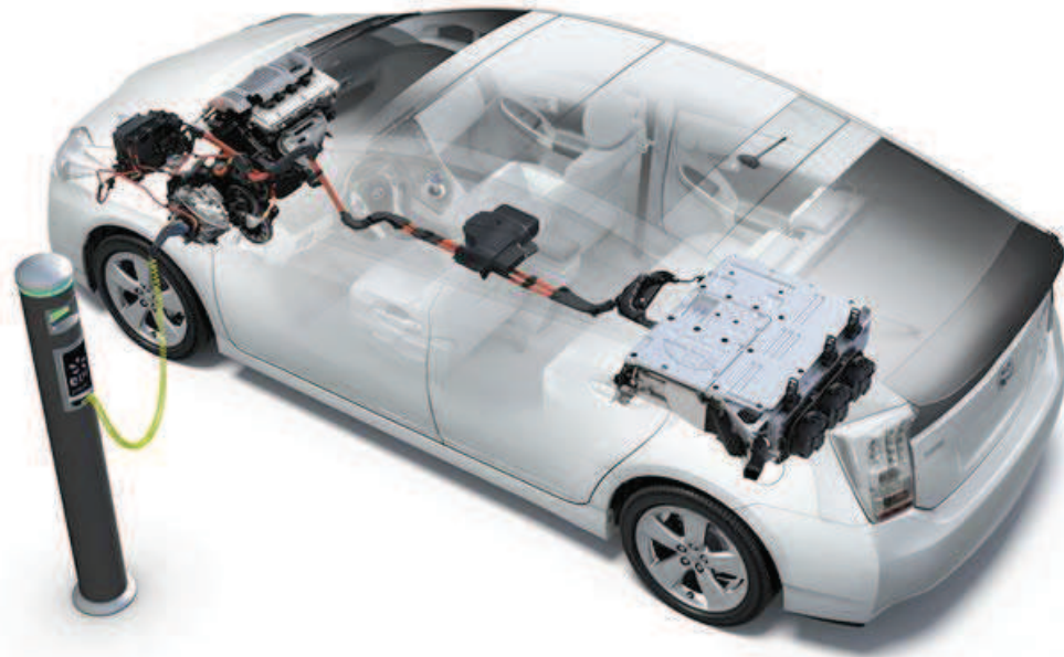
Figure 1.15 : Architecture Toyota Prius rechargeable.
