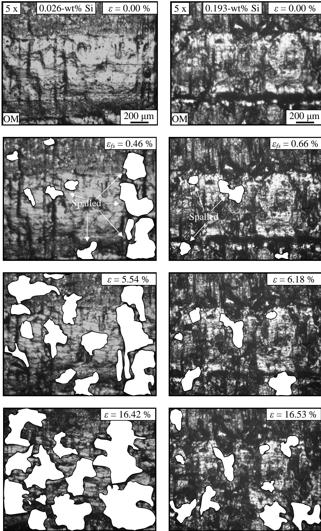
Figure 4.15: Evolution of scale failure on the as-received hot-rolled 0.026-wt% Si steel (left) and the as-received hot-rolled 0.193-wt% Si steel (right) as a function of imposed strain investigate by the macro-tensile test (strain rate = 0.83 \text{ s}^{-1} ).
