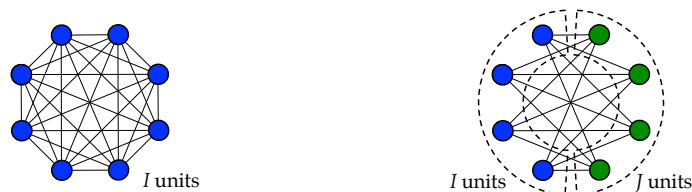
(a) Network of fully-connected units. (b) Bipartite structure of the restricted Boltzmann machine.
