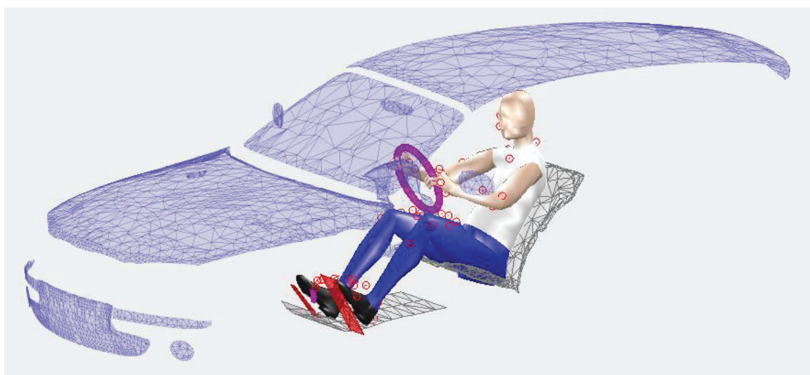
Figure 15: Reconstructed driving posture and recorded vehicle geometry. The markers attached to the body are also showed as well as their residual errors with respect to measured positions, characterized as a directed line from the center of each marker.
