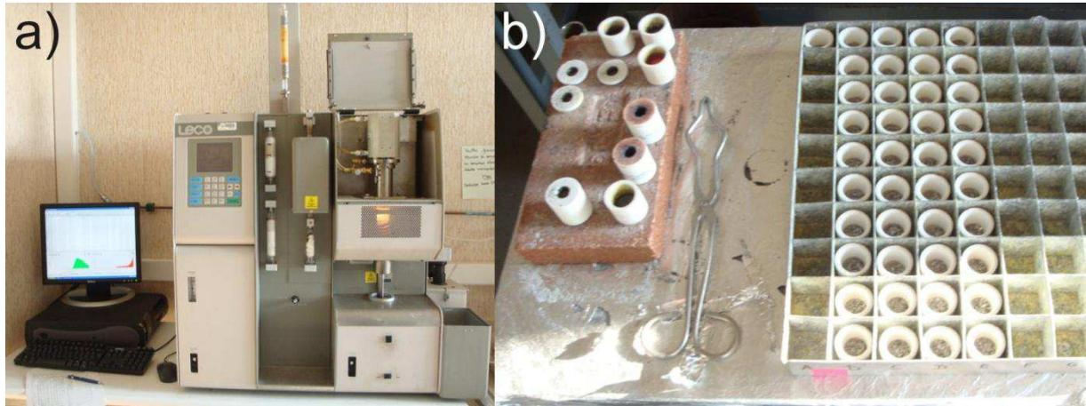
Fig. 3-5: Total and Organic Carbon analysis – a) Treated samples with HCl and b) LECO device
