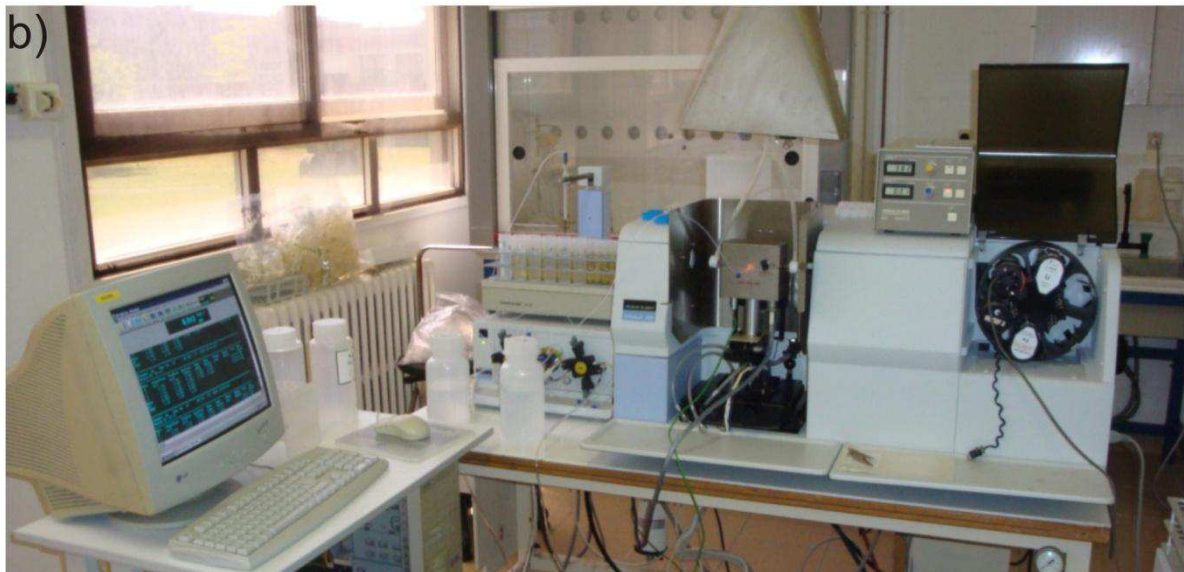
Fig. 3-8: Flow Injection Atomic Absorption Spectrophotometry, a) Schematic operation diagram of FIAS 300 (modified from Hineman, 2011) b) Measurement equipment at EPOC laboratory.
