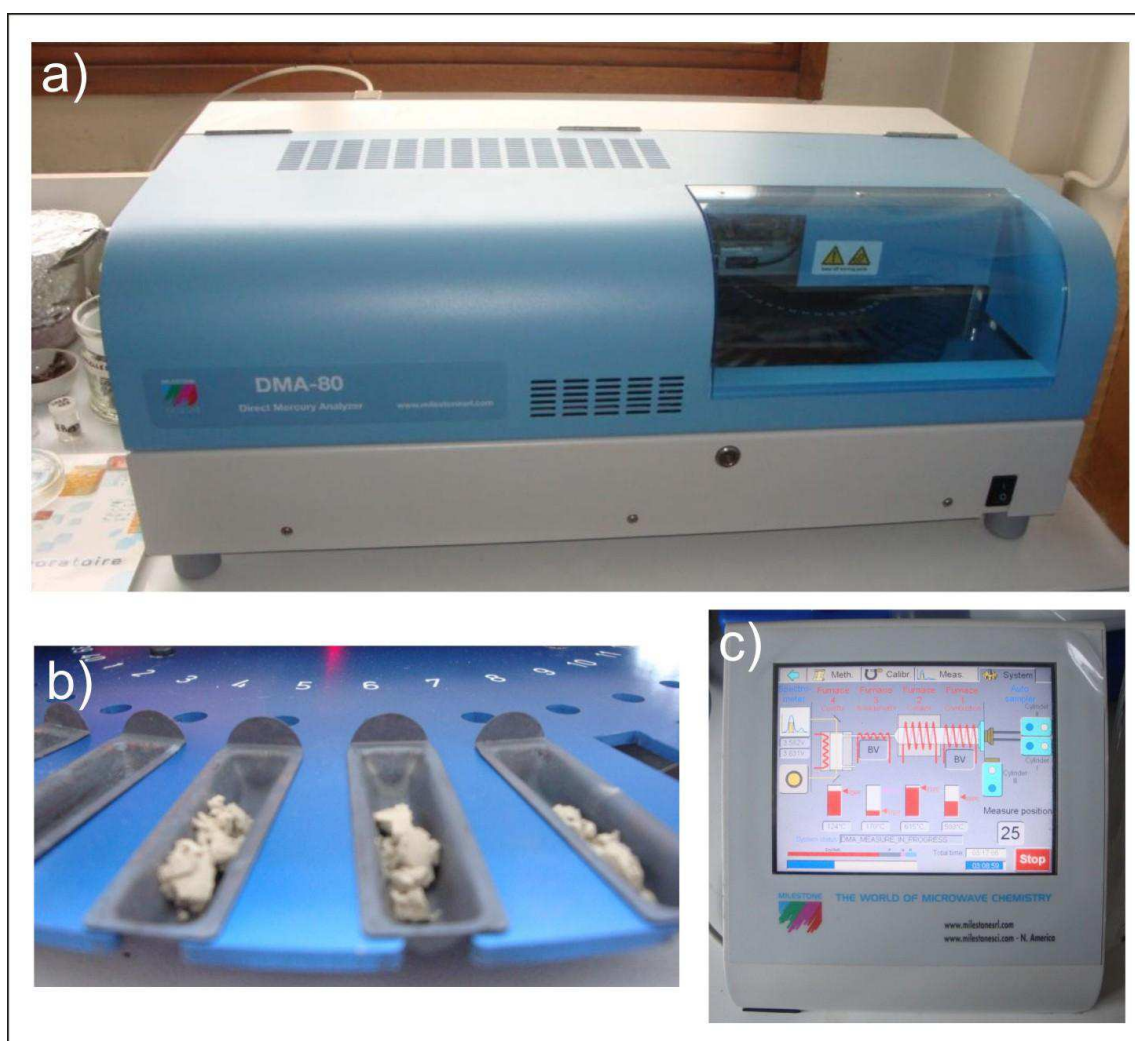
Fig. 3-7: Direct Mercury Analyzer (DMA) 80 MILESTONE – a) Analyzer device, b) Auto-sampler tray, c) Read-out terminal.
