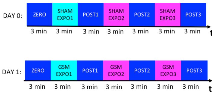
Figure 3-29: Time profile of the test protocols: sham exposure on day 0 and GSM exposure on day 1.
