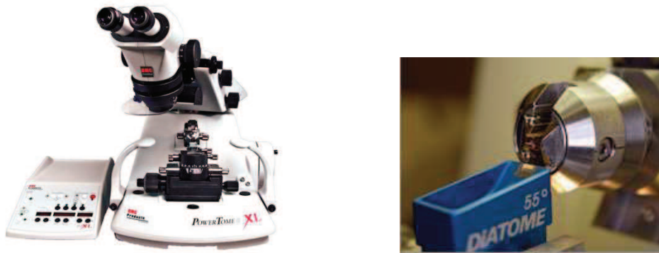
Figure 9 : Ultramicrotome PowerTome XL de RMC products (a) muni d'un couteau diamant (b)
