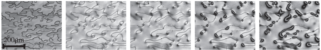
Figure 3.6: Temporal snapshots with steps of 400\mu s of the early dynamics in the biased nematic cell, from t = 0 (left) when a bias voltage of 15V is applied. Some of defect loops evolve in a random network of umbilics of alternate sign, others collapse.
