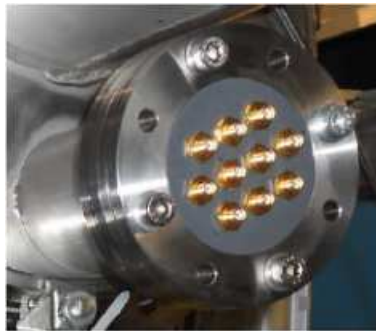
Figure 4.26: CF73 vacuum flange, that contains a 6 mm-thick isolating Trovidur bloc in which the 10 SMA vacuum feedthroughs are fixed. On the vacuum side, the SMA cables are enclosed in a plastic tube which is itself enclosed in an aluminum tube.
