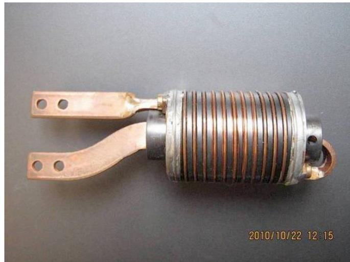
Figure 3-15 Coils with  $\text{MgB}_2$  wires for transport current measurement
