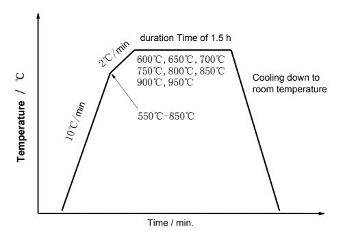
Figure 2-2 A temperature profile for the annealing of MgB<sub>2</sub> wires
