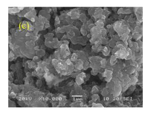
Figure 3-7 SEM pictures of MgB<sub>2</sub> wires at a magnification of 10000× times. a) 650 °C, b) 750 °C, and c) 850 °C
