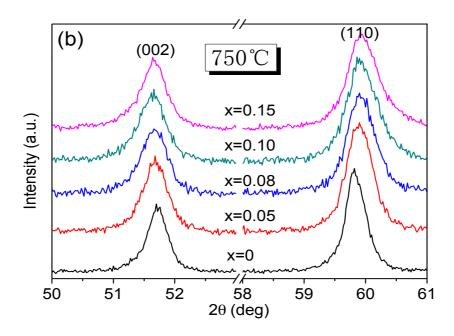
Figure 4-4 Comparison of (002) and (110) characteristics peak of MgB<sub>2-x</sub>(TiC)<sub>x</sub> wires
