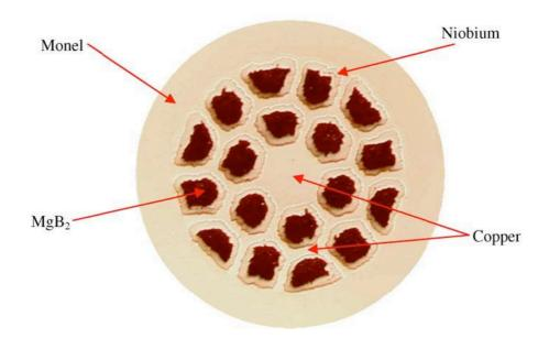
Figure 1-15 Cross section of typical 18+1 multifilament MgB<sub>2</sub> wire fabricated by Hyper Tech Research
