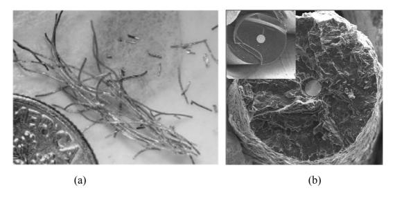
Figure 1-10 MgB<sub>2</sub> wire fabricated by Mg infiltration method [77]
