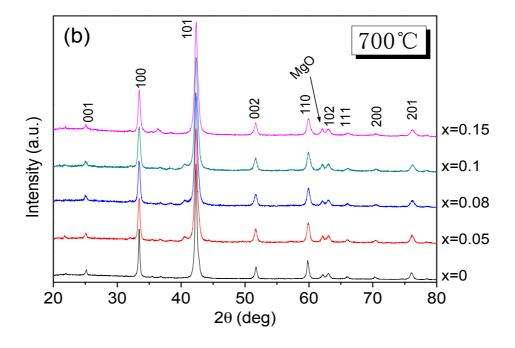
Figure 4-2 XRD patterns of MgB<sub>2-x</sub>(TiC)<sub>x</sub> ( x = 0, 0.05, 0.08, 0.1, 0.15) wires heat treated at 650 °C (a) and 700 °C (b).
