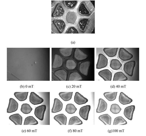
Figure 5-10 Optical microscopy image (a) and Magneto-optical image (b-g) of 6-filamentary MgB<sub>2</sub> wires at 6 K with a perpendicular applied field from 0 to 100 mT
