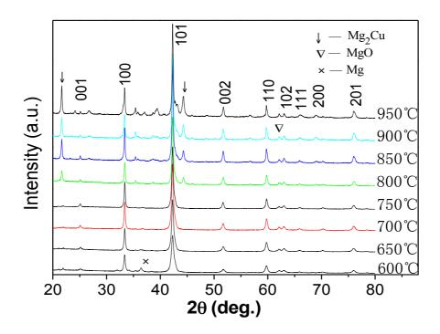
Figure 3-1 XRD patterns of superconducting cores of MgB<sub>2</sub> wires with various sintering temperatures
