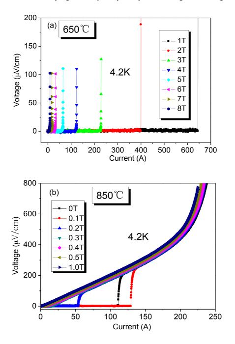
Figure 3-13 Voltage-Current Curves of the MgB<sub>2</sub>/Nb/Cu wires heat treated at (a) 650 °C and (b) 850 °C at 4.2K
