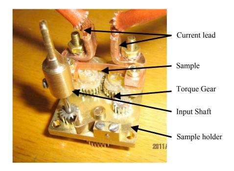
Figure 5-5 Bending strain measurement holder
