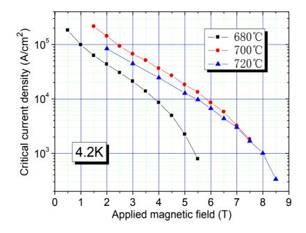
Figure 3-16 Transport  $J_c$  as a function of the field for MgB<sub>2</sub> coil at 4.2K
