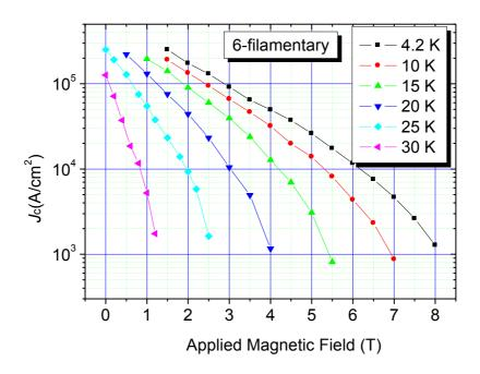
Figure 5-13 Transport  $J_c$  as a function of magnetic field on 6-filamentary  $MgB_{1.92}(TiC)_{0.08}$  wires at different temperature
