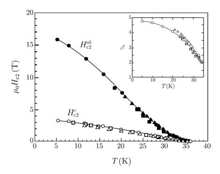
Figure 1-6 Temperature dependence of upper critical field of MgB<sub>2</sub> single crystal.
