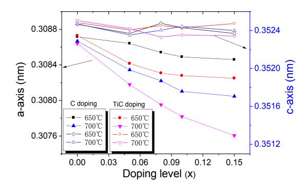
Figure 4-5 Crystal parameters of MgB<sub>2</sub>/Nb/Cu wires with TiC and C doping
