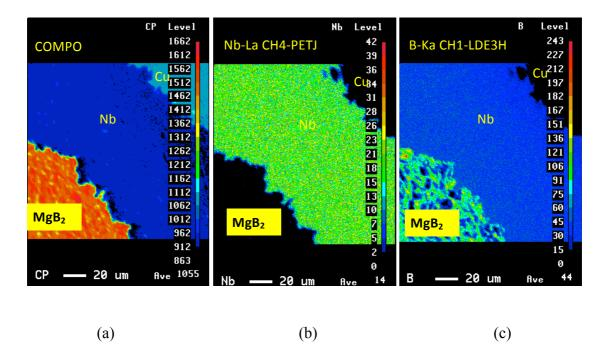
Figure 3-24 EPMA element maps for niobium (b) and boron (c) of the MgB<sub>2</sub>/Nb/Cu wires heat treated at 900 °C
