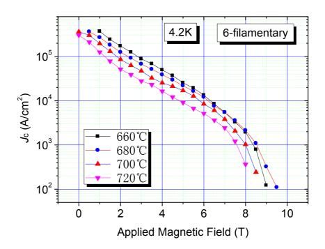
Figure 5-12 Transport  $J_c$  as a function of magnetic field on 6-filamentary  $MgB_{1.92}(TiC)_{0.08}$  wires at 4.2 K with the field up to 10 T
