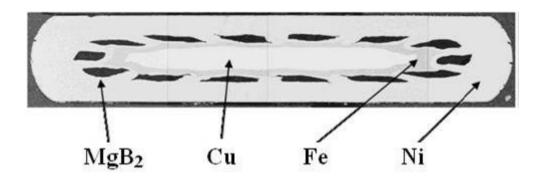
Figure 1-14 Transverse cross section of the MgB<sub>2</sub> superconducting tape fabricated by Columbus Superconductors
