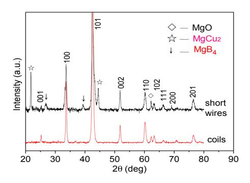
Figure 3-5 XRD patterns of short sample and long wires heat treated at 800 °C
