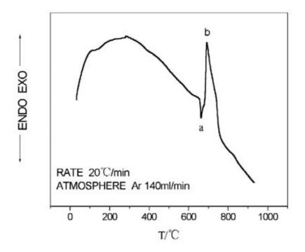
Figure 1-8 DTA curve of Mg:B = 1:2 mixture [22]
