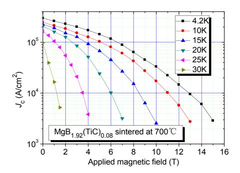
Figure 4-18 Transport  $J_c$  of MgB<sub>2-x</sub>(TiC)<sub>x</sub> with the field up to 16 T at different testing temperatures.
