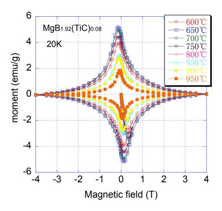
Figure 4-14 M-H curves of the MgB<sub>1.92</sub>(TiC)<sub>0.08</sub> wires heat treated at different temperatures
