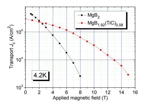
Figure 4-17 Transport  $J_c$  of MgB<sub>2</sub> and MgB<sub>1.92</sub>(TiC)<sub>0.08</sub> at 4.2K with the magnetic field up to 16 T
