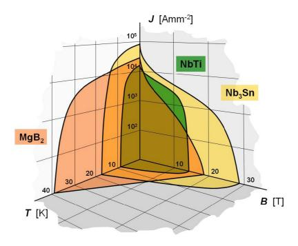
Figure 1-9 Critical surfaces of MgB2, NbTi and Nb3Sn  $^{[23]}$
