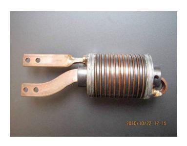
Figure 3-15 Coils with MgB<sub>2</sub> wires for transport current measurement
