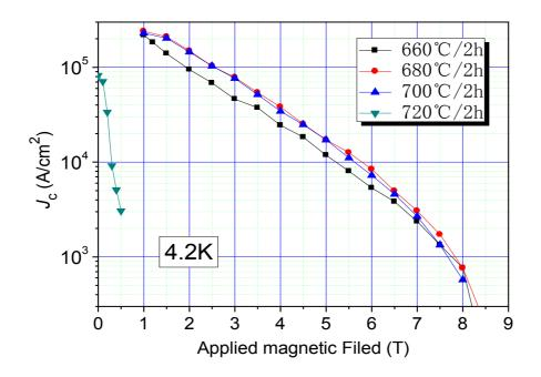
Figure 3-14 Transport  $J_c$  of short MgB<sub>2</sub>/Nb/Cu wires with different sintering temperatures at 4.2K
