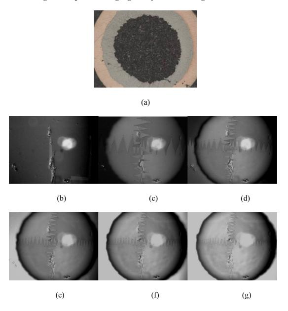
Figure 3-19 Magneto-optical image of MgB<sub>2</sub> wires heat treated at 650 °Cunder the magnetic fields from zero to 100 mT
