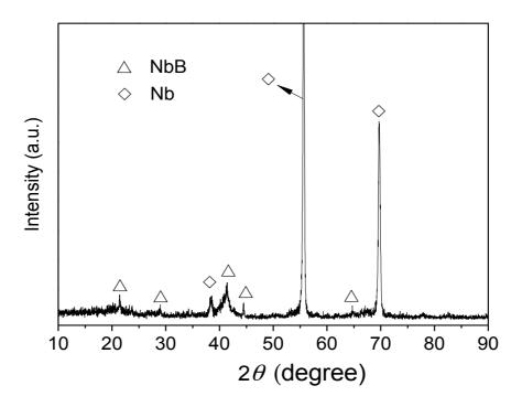
Figure 3-23 XRD pattern of MgB<sub>2</sub>-Nb interface
