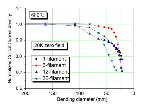
Figure 5-6 Critical current declines dependent on the bending radius of different filamentary wires
