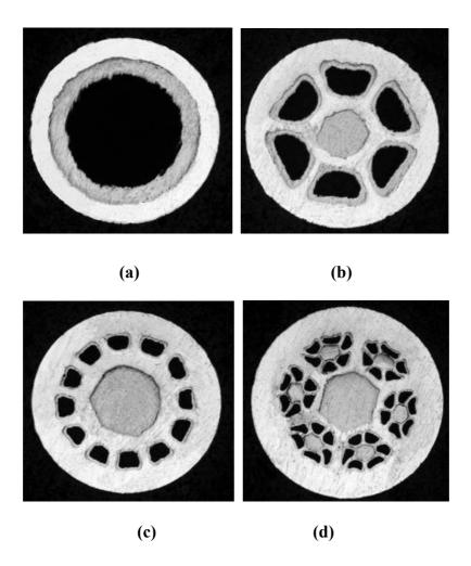
Figure 5-1 Cross section of the MgB<sub>1.92</sub>(TiC)<sub>0.08</sub>/Nb/Cu wires with different filament. (a) mono-filamentary, (b) 6-filamentary, (c) 12-filamentary and (d) 36-filamentary
