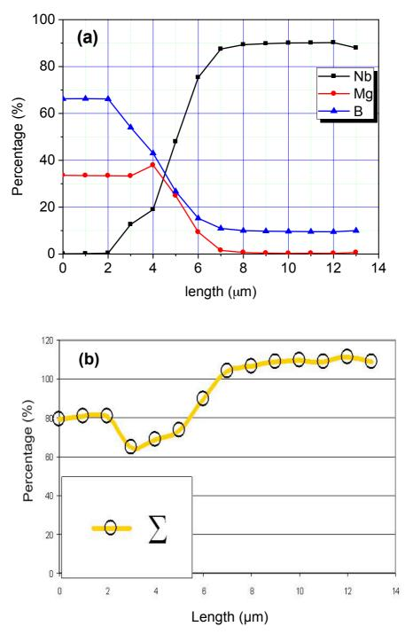
Figure 3-25 EPMA line scanning of MgB2-Nb interface in MgB2 wires heat treated at  $900\ ^{\circ}\text{C}$
