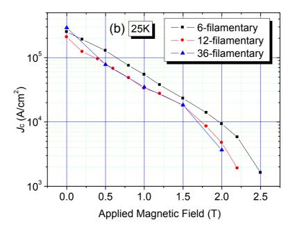
Figure 5-11 Transport  $J_c$  as a function of magnetic field on MgB<sub>1.92</sub>(TiC)<sub>0.08</sub> wires with different filaments
