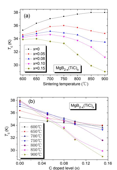
Figure 4-10 Critical temperature as a function of doping content on  $MgB_{1.92}(TiC)_{0.08}$  wires heat treated at different temperatures
