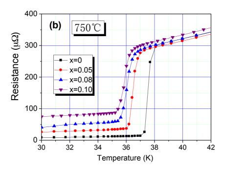
Figure 4-11 Resistance depend on the temperature of  $MgB_{2-x}(TiC)_x$  wires heat treated at 700 °C (a) and 750 °C(b).
