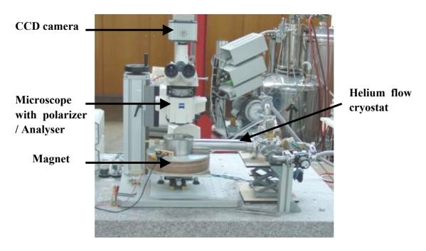
Figure 2-5 Photograph of Magneto Optical Equipment
