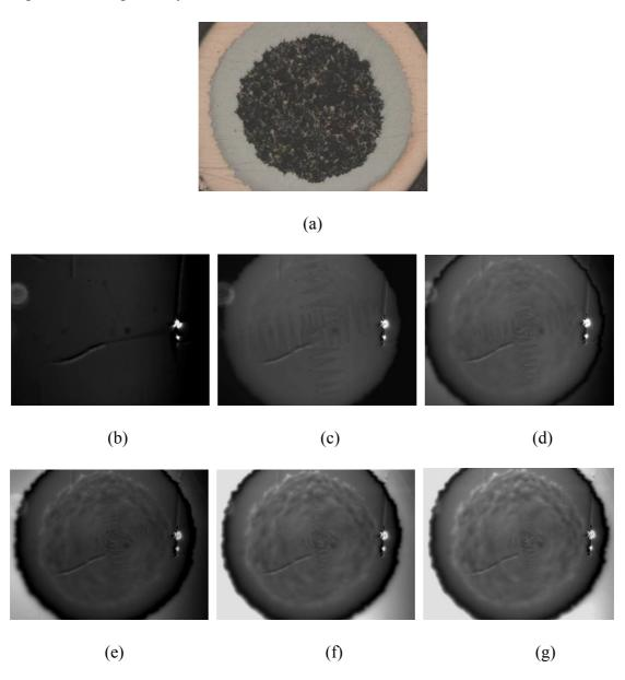
Figure 3-20 Magneto-optical image of MgB<sub>2</sub> wires heat treated at 800 °C under the magnetic fields from zero to 100 mT
