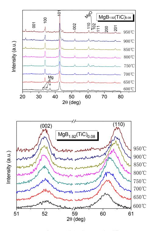
Figure 4-6 XRD pattern of  $MgB_{1.92}(TiC)_{0.08}$  heat treated at different temperatures
