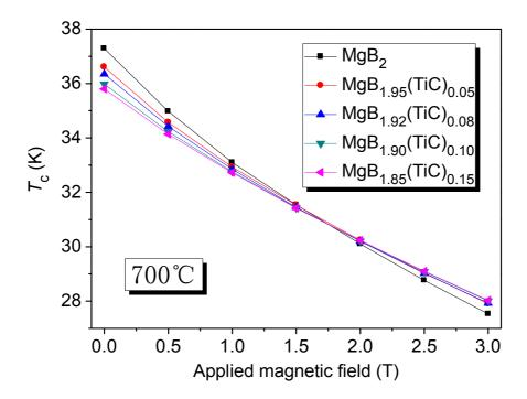
Figure 4-13 T<sub>c</sub> verses magnetic field of MgB<sub>2</sub> wires with TiC doping
