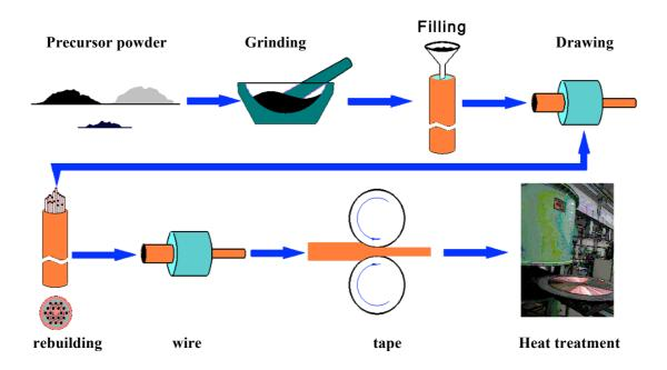
Figure 2-1 Schematics of the *in-situ* PIT process for the fabrication of multi-filamentary MgB<sub>2</sub>/Nb/Cu wires and tapes
