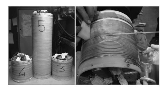
Figure 1-17 Photograph of MgB<sub>2</sub> SFCL prototypes (left) and detail of electrical connections (right)<sup>[104]</sup>
