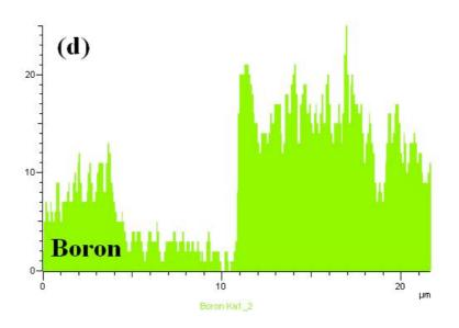
Figure 3-17 EDS Analysis of the interface layer between MgB<sub>2</sub> and Nb
