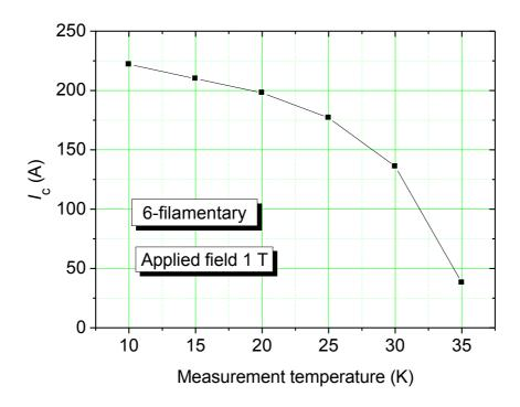
Figure 5-14 Critical current  $I_c$  as a function of temperature on 6-filamentary  $MgB_{1.92}(TiC)_{0.08}$  wire
