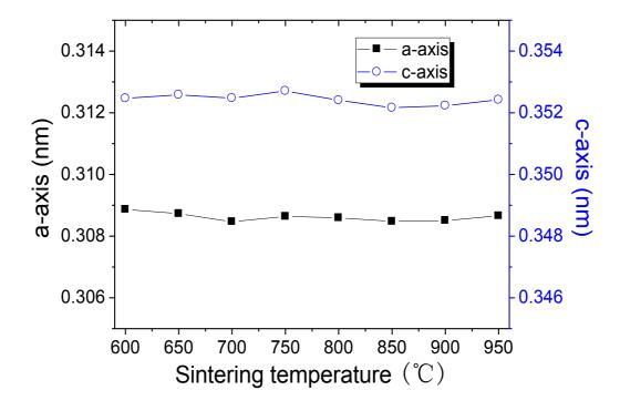
Figure 3-3 Lattice parameters of MgB<sub>2</sub> wires heat treated at different temperature
