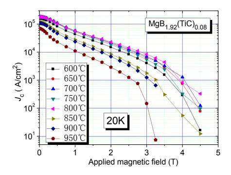
Figure 4-15 Magnetic  $J_c$  versus applied field for the MgB<sub>1.92</sub>(TiC)<sub>0.08</sub> wires at different temperatures
