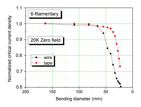
Figure 5-7 Comparison of the  $J_c$  degradation with the bending of 6-filamentary wires and tapes
