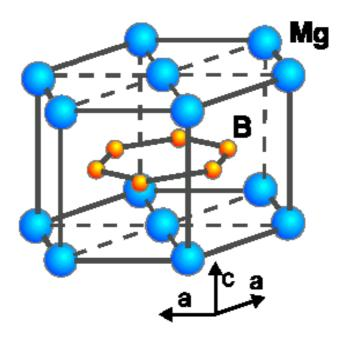
Figure 1-4 Hexagonal (AlB<sub>2</sub>-type) crystal structure of MgB<sub>2</sub>
