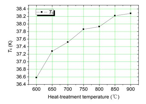
Figure 3-11 Relationship between the heat treatment temperature and  $T_c$
