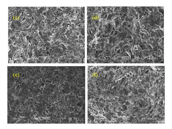
Figure 3-6 Microstructure of MgB<sub>2</sub> wires heat treated at various temperature of a) 650 °C, b) 700 °C, c) 750, d) 800 °C, e) 850 °C, and f) 900 °C
