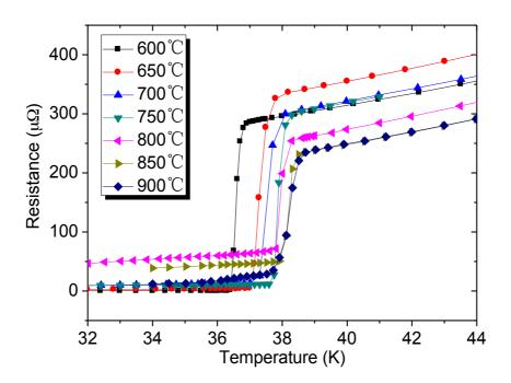
Figure 3-10 Resistance vs measurement temperature curves of MgB<sub>2</sub> wire heat treated at different temperatures
