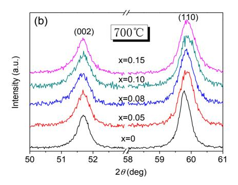
Figure 4-3 Comparison of (002) and (110) characteristics peak of MgB<sub>2-x</sub>C<sub>x</sub> wires
