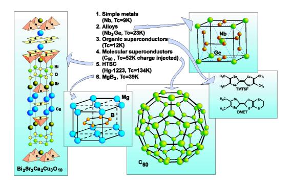
Figure 1-5 Comparison of the crystal structures of MgB<sub>2</sub> and some others practical superconductors
