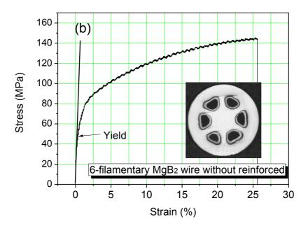
Figure 5-2 Tensile stress vs strain curve of 6-filamentary MgB<sub>2</sub> wires with (a) or without (b) Nb reinforcement after heat treated at 680 °C for 1.5 hours.
