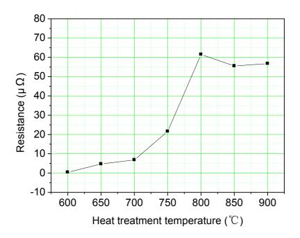
Figure 3-12 Residual resistance just below the transition point as a function of heat treatment temperature
