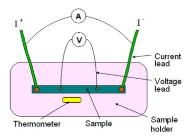
Figure 2-8 Schematic diagram of standard Four-probe method for the  $MgB_2$  wires
