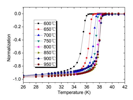
Figure 3-8 Magnetization curves of MgB<sub>2</sub> wires with various sintering temperatures
