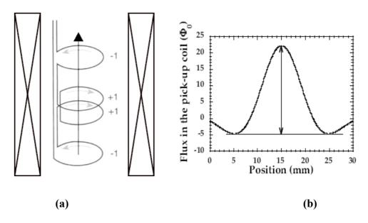
Figure 2-6 Design of the pick-up coil with the superconducting coil (a) and magnetic flux in the coil versus the position of the sample (b)
