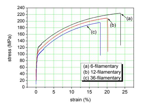
Figure 5-3 Room-temperature stress-strain curves of 6-, 12- and 36-filamentary MgB<sub>2</sub>/Nb/Cu wires
