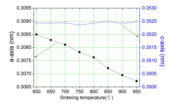
Figure 4-7 Lattice parameter of  $MgB_{1.92}(TiC)_{0.08}$  wires heat treated at different temperatures
