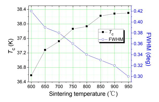
Figure 3-4 The FWHM value of MgB<sub>2</sub> wires heat treated at different temperature
