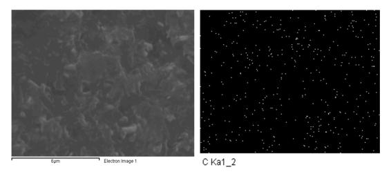
Figure 4-8 Second electron image of MgB<sub>1.92</sub>(TiC)<sub>0.08</sub> wires heat treated at 700 °C
