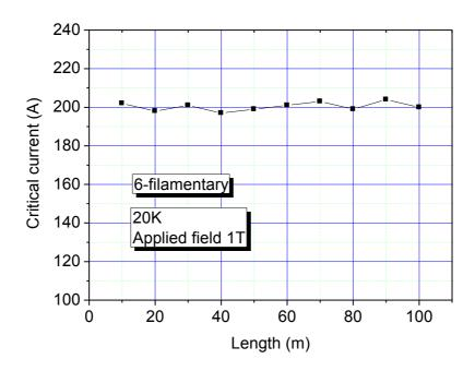
Figure 5-16 Homogeneity of critical current of MgB<sub>2</sub> wire (20K, 1T)
