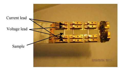
Figure 2-7 The sample holder for resistance measurement
