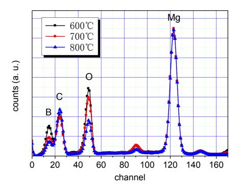
Figure 3-18 EDS analysis of MgB<sub>2</sub> superconductor filament
