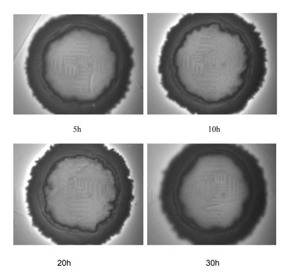
Figure 3-21 MOI of the samples heat-treaded at 800 °C for different time from 5 hours to 30 hours
