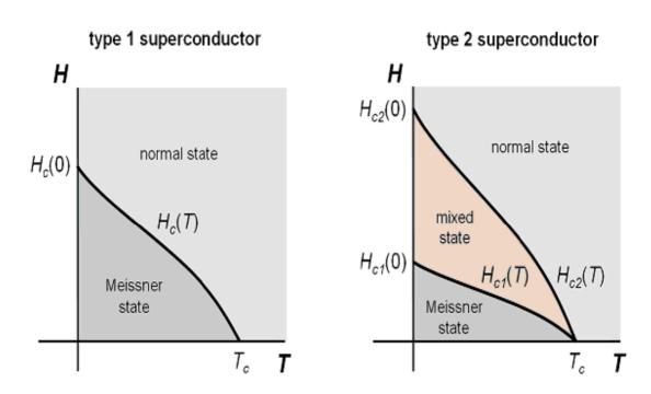
Figure 1-3 Difference between type and type superconductor
