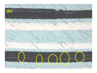
Figure 5-9 Cracks in mono-filamentary (a) and 6-filamentary (b) MgB $_2$  wires heat treated at 700  $^{\circ}$ C
