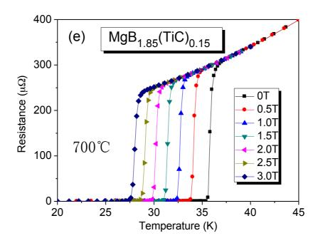
Figure 4-12 Field dependence of the R-T curves of the MgB<sub>2-x</sub>(TiC)<sub>x</sub> wires in 3.0 T, 2.5 T, 2.0 T, 1.5 T, 1.0 T, 0.5 T and 0 T from left to right in perpendicular fields
