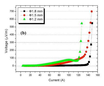
Figure 5-15 Critical current measurement of 100 meter MgB<sub>2</sub>/Nb/Cu wires
