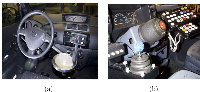
Figure 1.3 – Examples of mini steering wheel (a) and joystick (b), provided by the Handi-Mobil manufacturer. These adaptation mechanisms are used in case of bilateral disabilities.
