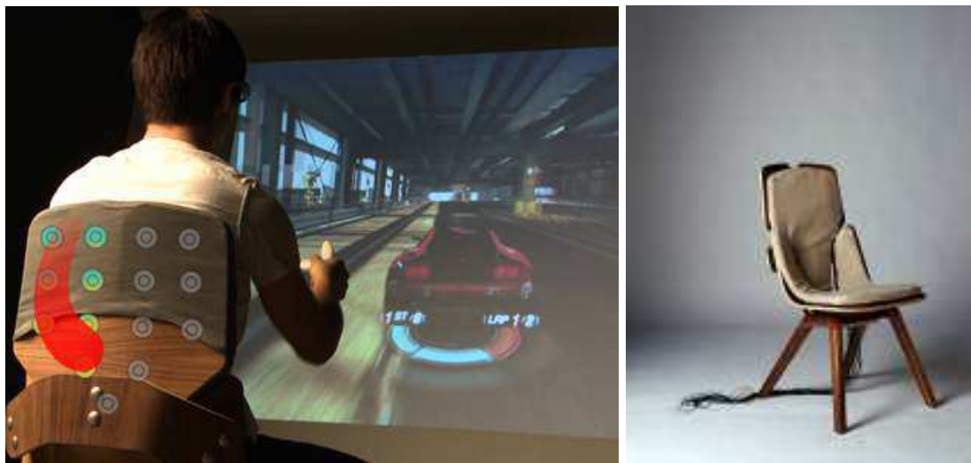
Figure 2.12: Haptic seat. Seat embedding an array of vibrotactile actuators [IP11].
