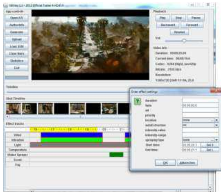
Figure 2.5: User-oriented graphical authoring tools - SEVino [WRTH12]. Haptic effects can be defined and synchronized to a video.
