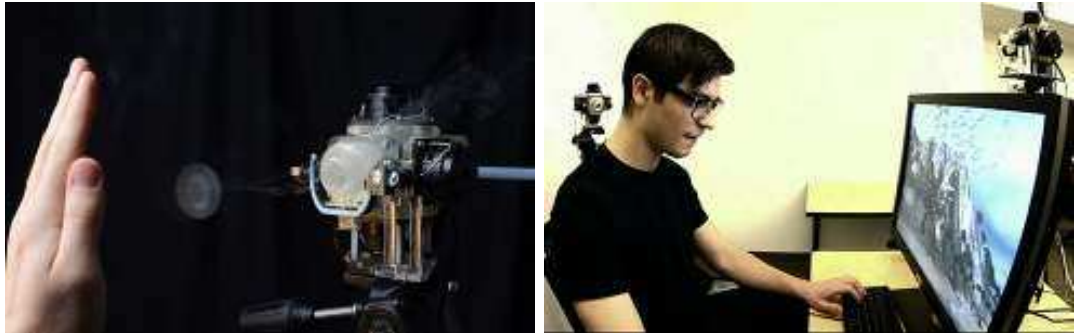
Figure 2.11: Desktop haptic device. The AIREAL, a contact free tactile interface [SPGI13].
