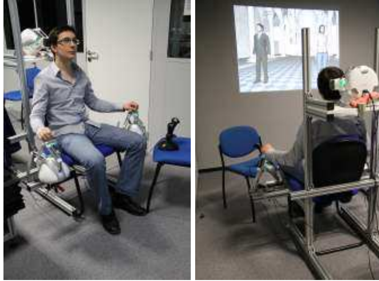
Figure 6.4: Experimental Setup, front view (left) and back view (right). The participant experiences haptic effects while watching a video.
