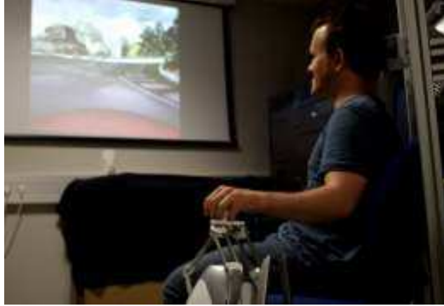
Figure 3.4: The user, comfortably installed on our device, is experiencing passive navigation enhanced by a haptic effect of motion.
