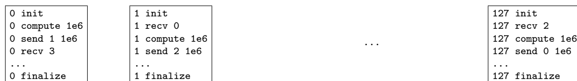
Figure 3.2: Example of a split time-independent trace corresponding to a larger application execution with 128 processes.
