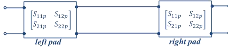
Figure 3.8 Two port network of the thru de-embedding test structure
