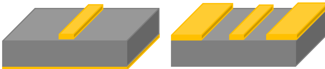
Figure 1.5 Generic view of 1) left side: microstrip line 2) right side: coplanar waveguide. They are potential platforms for characterizing nanowires, in which the central conductor can be replaced by the intended test sample.
