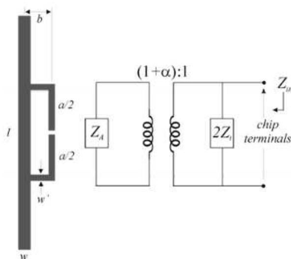
Figure 2.12 – La configuration T-match et le circuit equivalent [2.13]
