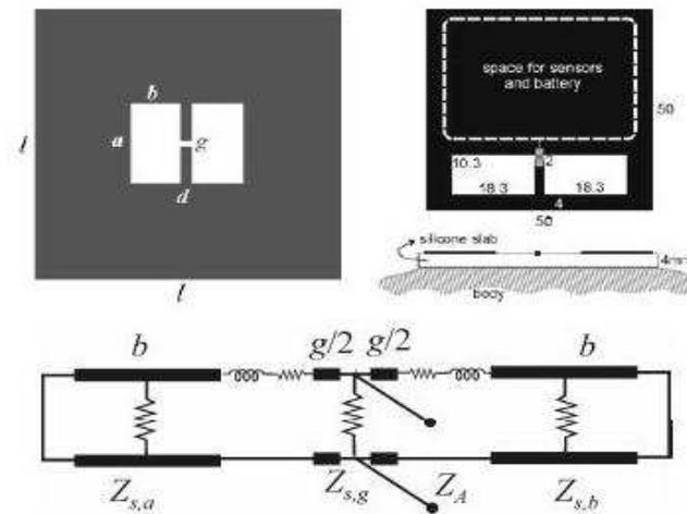
Figure 2.15 – La configuration de Nested-slot [2.13]
