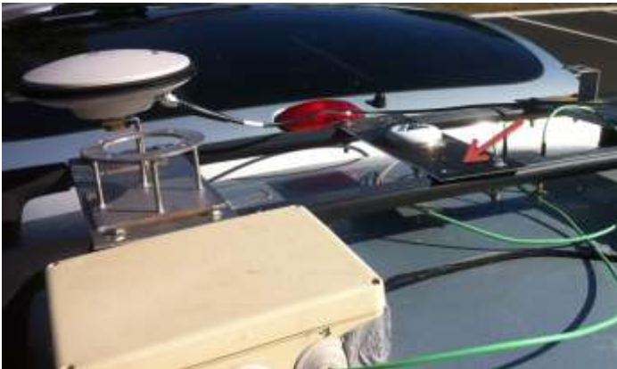
Figure 5.24 Picture of the vehicle roof configuration. The Novatel geodetic antenna connected to the SPAN module can be seen on the left, while the place where the antenna was magnetically stucked is pointed by the red arrow.
