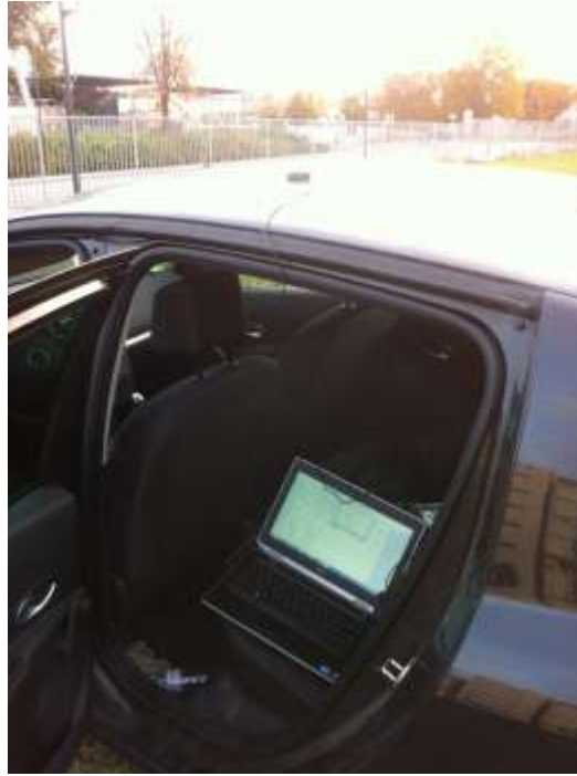
Figure 2.17 Patch antenna stuck to the roof of the car on the surveyed reference point
