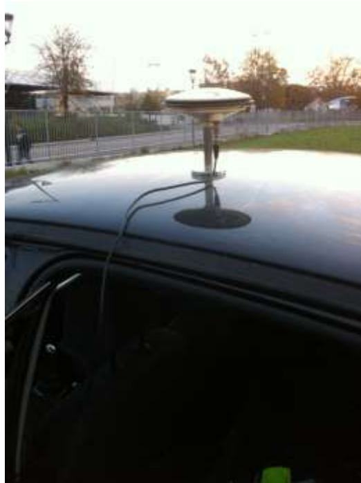
Figure 2.15 Surveyed equipment to determine the position of the reference point on the top of the car
