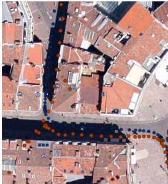
Figure 6.9 Example of Kalman filter propagation leading to large position error. Orange dots indicate estimated position and blue dots indicate reference trajectory. The vehicle goes from the top of the picture to the bottom right
