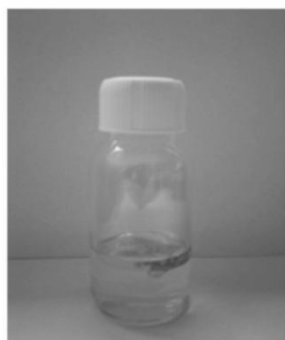
Figure 12. Solubility tests of the network obtained via Diels-Alder reaction in TCB after 48h.
