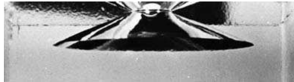
Figure 5.29: The hertzian cone, experimentally observed. (Taken from [150]).
