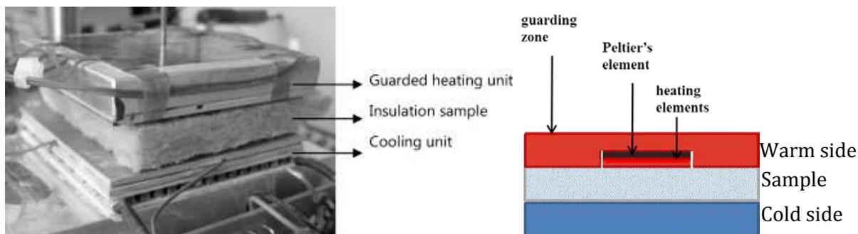
**Figure 68: Home-made (EMPA) experimental device used for the evaluation of thermal conductivity of foams.**<sup>227</sup>
