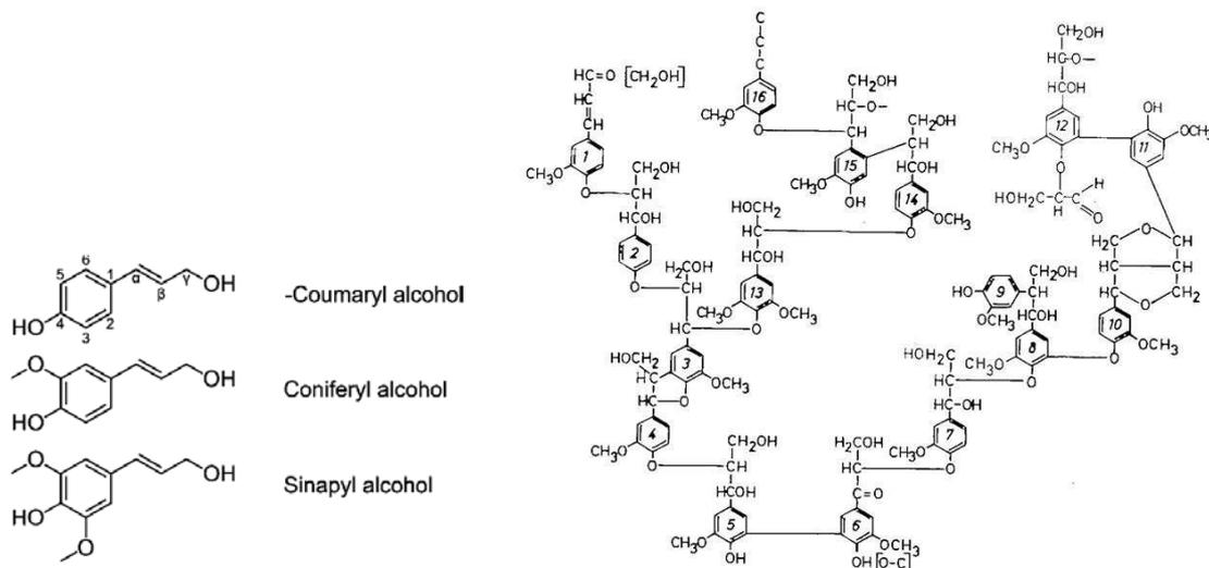
**Figure 4: The three fundamental lignin monomer precursors<sup>20</sup> (left) and a model of lignin structure<sup>29</sup> (right).**
