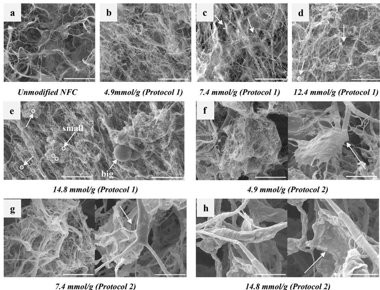
**Figure 32: SEM micrographs of unmodified NFC (a) and NFC treated with MTMS, according to Protocol 1 (b-e) or Protocol 2 (f-h) (Scale bar is 10 μm). Results with various [MTMS]<sub>i</sub> are presented.**
