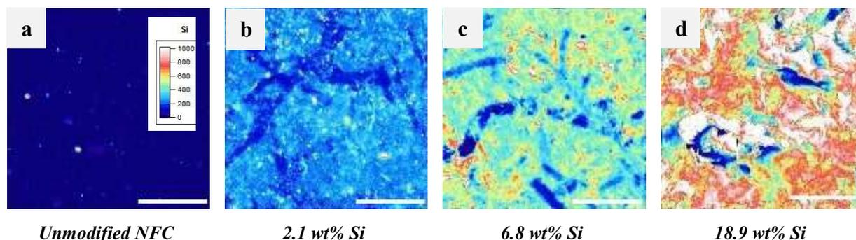
**Figure 55: WDX Si mapping of unmodified NFC foam (a) and silylated NFC foams prepared at different [MTMS]<sub>i</sub> according to *Protocol 2*'. (Scale bar is 100  $\mu\text{m}$ )**
