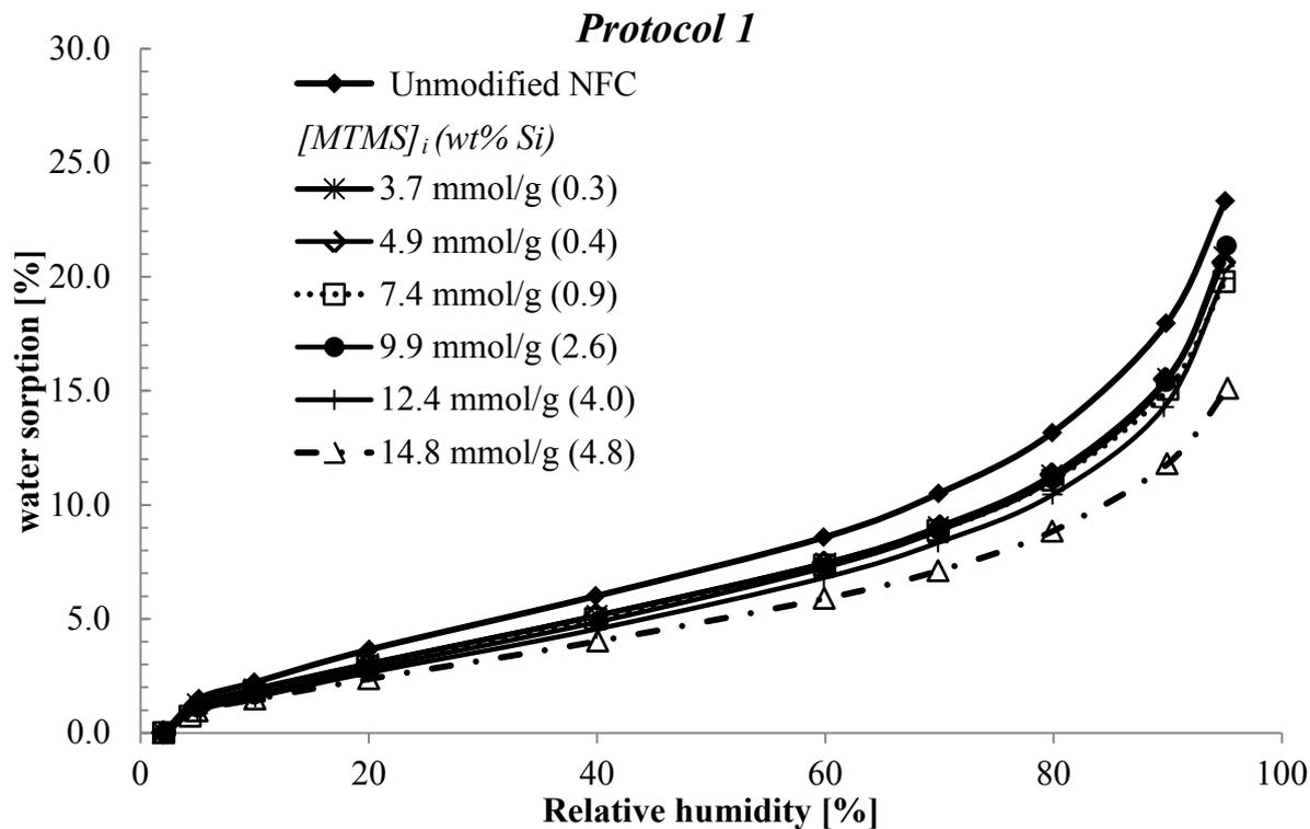
**Figure 39: Water sorption isotherms of unmodified NFC and NFC treated at different  $[MTMS]_i$  according to *Protocol 1* ( $T = 23\text{ }^\circ\text{C}$ ).**
