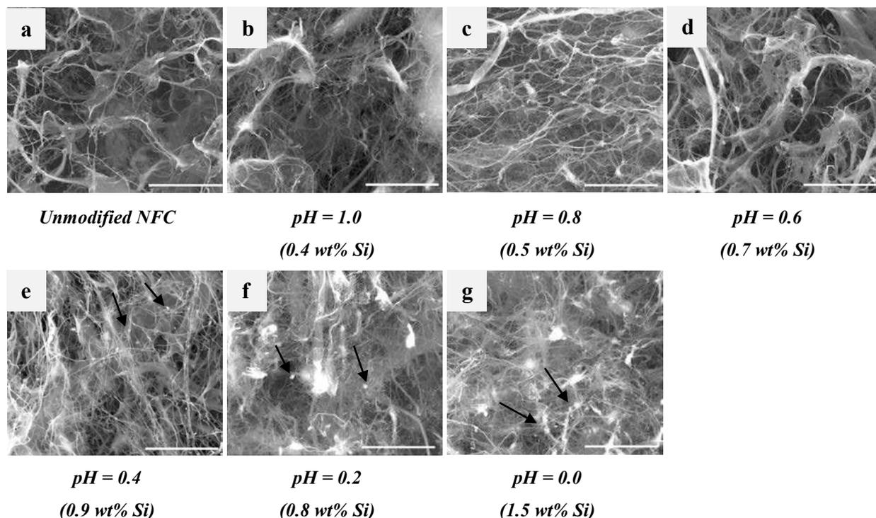
**Figure 20: SEM micrographs of unmodified NFC (a) and NFC treated with MTMS (Protocol I) in the pH range 1-0 (b-g). (Scale bar is 10  $\mu\text{m}$ ).**
