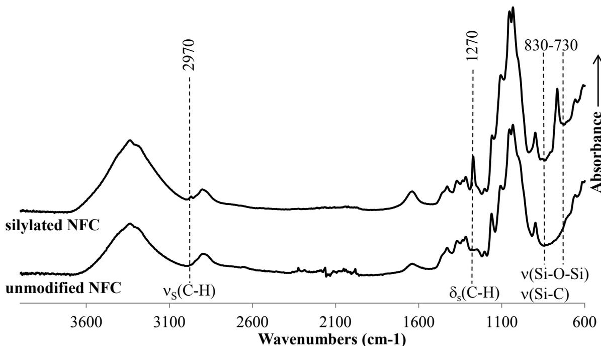
**Figure 14:** Example of FTIR spectra obtained after analysis of unmodified and MTMS-treated NFC (*Protocol 1*) samples.  $\nu$ , stretching vibration;  $\delta$ , in-plane bending,  $\gamma$ , out-of-plane bending.
