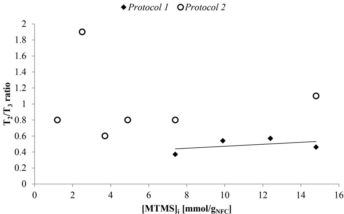
**Figure 31: Evolution of the ratio of the peaks area at -56 and -65 ppm ( $T_2/T_3$  ratio) as a function of  $[MTMS]_i$ .**
