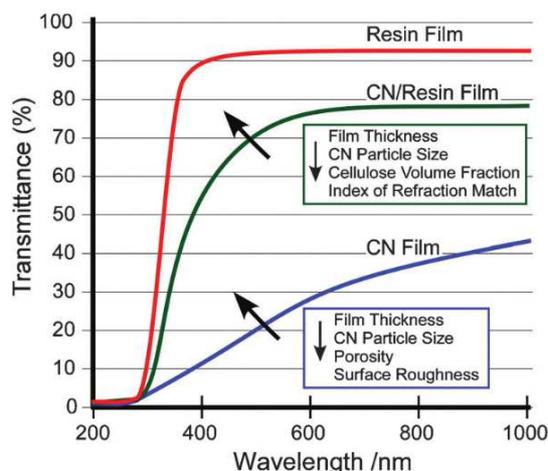
**Figure 10: Factors impacting the light transmittance of CN/resin composites.<sup>39</sup> (CN refers to different types of nanocelluloses, such as NFC and CNC)**
