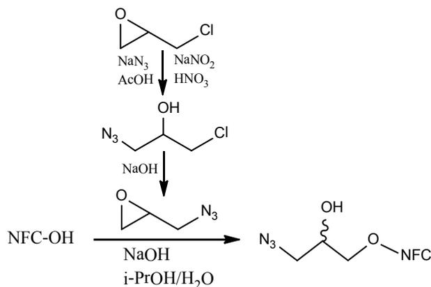
**Scheme 8: Etherification of NFC with 1-azido-2,3-epoxypropane.**<sup>134</sup>
