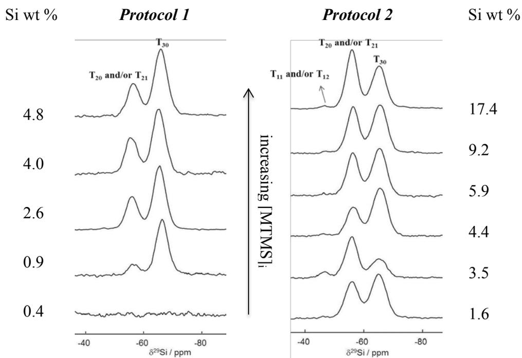
**Figure 30:  $^{29}\text{Si}$  CP-MAS solid state NMR spectra of MTMS-treated NFC prepared at different  $[\text{MTMS}]_i$  (Protocol 1 & 2).**
