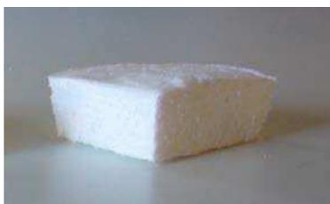
**Figure 11: Image of NFC foam prepared by the freeze-drying method.**<sup>104</sup>
