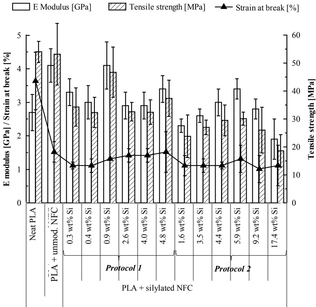
**Figure 51: Elastic modulus (E), tensile strength ( $\sigma$ ) and strain of break ( $\epsilon$ ) of PLA composites containing 10 % NFC treated at different [MTMS]<sub>i</sub> according to *Protocol 1* or *Protocol 2*.**
