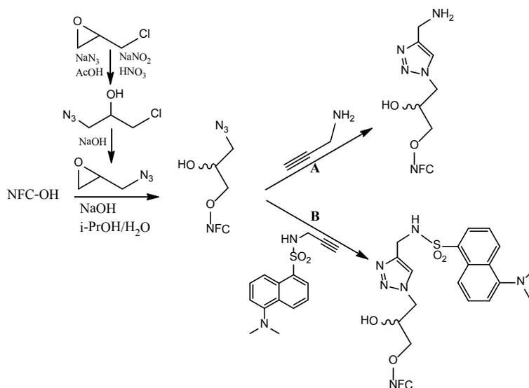
**Scheme 12: Functionalization of NFC by Copper-Catalyzed Azide Alkyne Cycloaddition.**<sup>134</sup>
