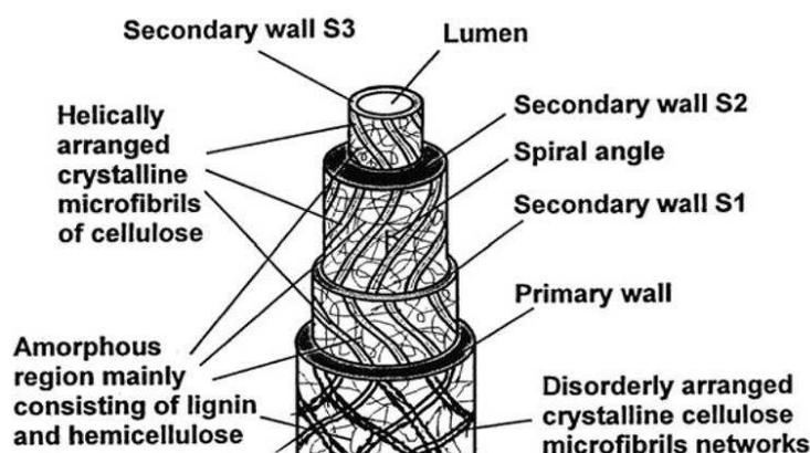
**Figure 6: Structural constitution of a plant fibre cell.**<sup>18</sup>
