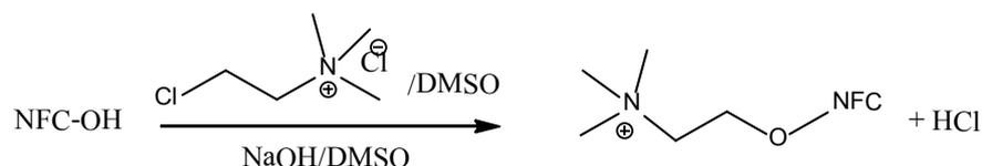
**Scheme 6: Cationic functionalization of NFC with choline chloride.**<sup>132</sup>
