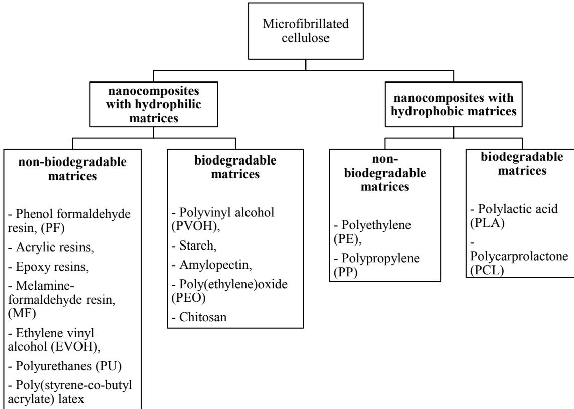
**Figure 9: Classification of nanocelluloses reinforced polymer composites, summarized by Siró et al.<sup>7</sup>**
