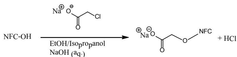
**Scheme 5: Carboxymethylation of NFC with chloroacetic acid sodium salt**
