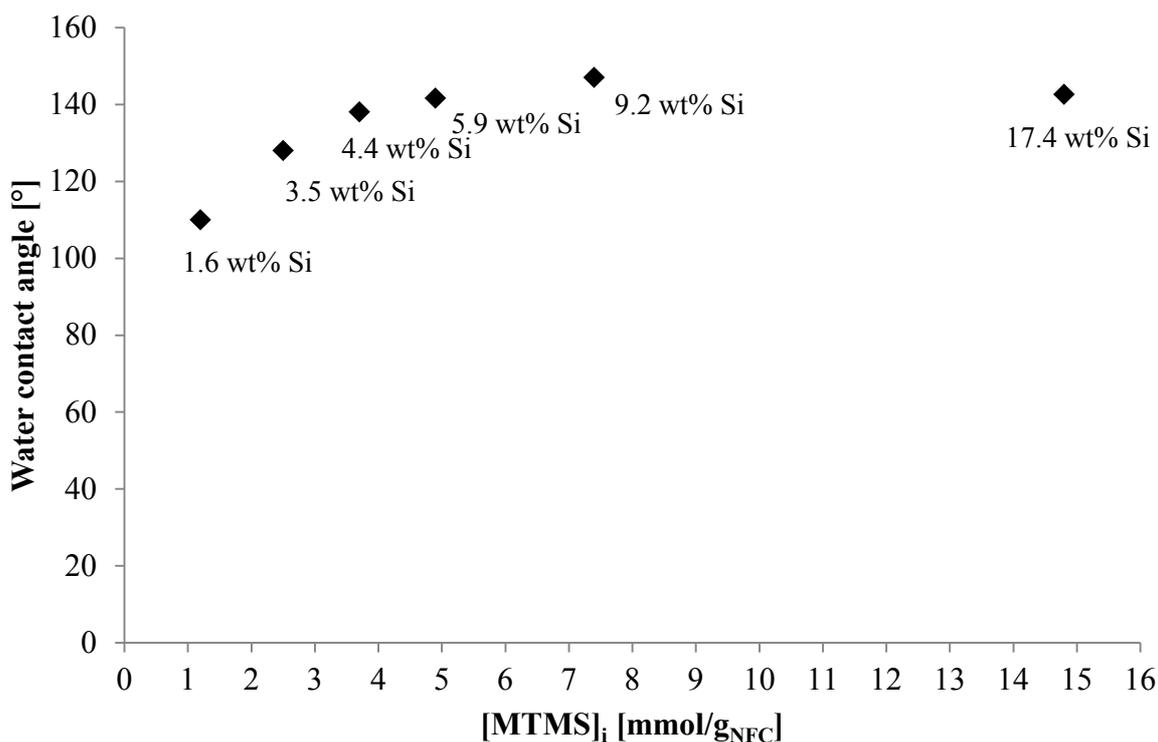
**Figure 38: Water contact angle (WCA) values at the surface of NFC treated at different [MTMS]<sub>i</sub> with *Protocol 2*.**
