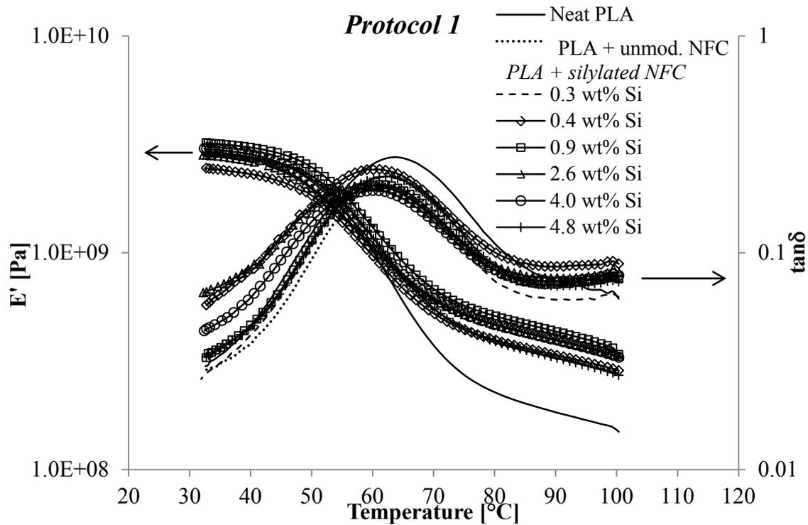
Figure 49: Storage moduli ( $E'$ , left-side Y-axis) and damping factor ( $\tan\delta$ , right-side Y-axis) of PLA composites containing 10 % NFC treated at different  $[MTMS]_i$  (*Protocol 1*)
