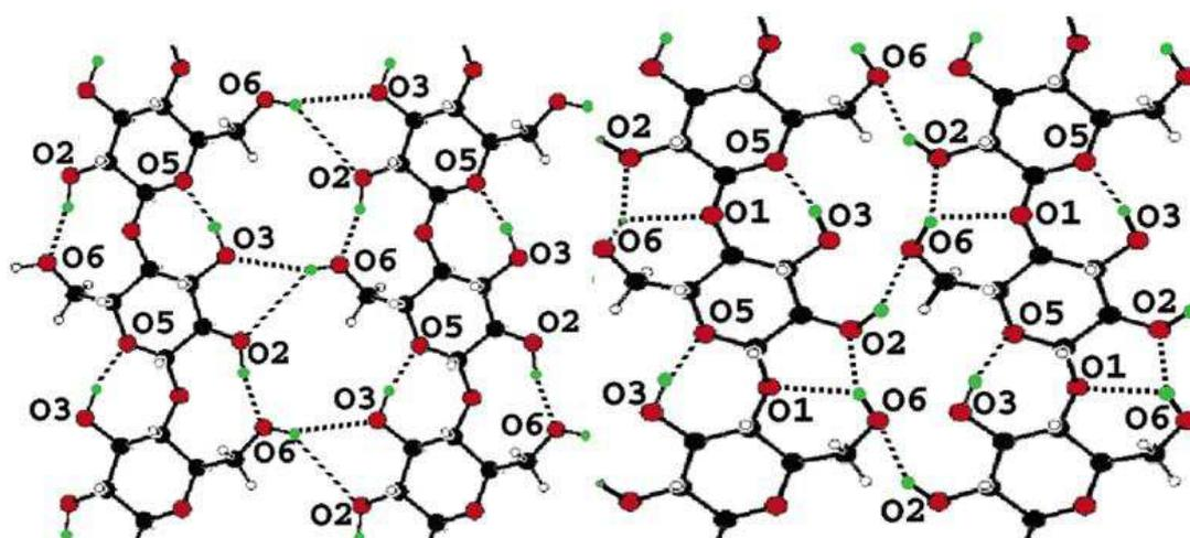
**Figure 2: Schematic representation of hydrogen bonds in cellulose I $\beta$ .**<sup>23</sup> Black: Carbon, red: Oxygen, white: hydrogen of methyl group, green: hydrogen of hydroxyl group; dotted line: hydrogen bonds. Only the oxygen atoms involved in hydrogen bonding are labelled.
