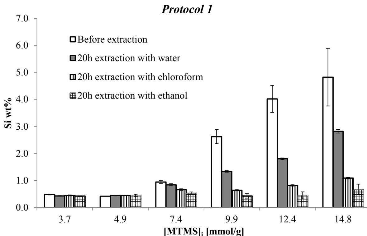
**Figure 34: Evolution of the Si content in MTMS-treated NFC prepared at different [MTMS]<sub>i</sub> (*Protocol 1*), before and after extraction with water, chloroform and ethanol.**
