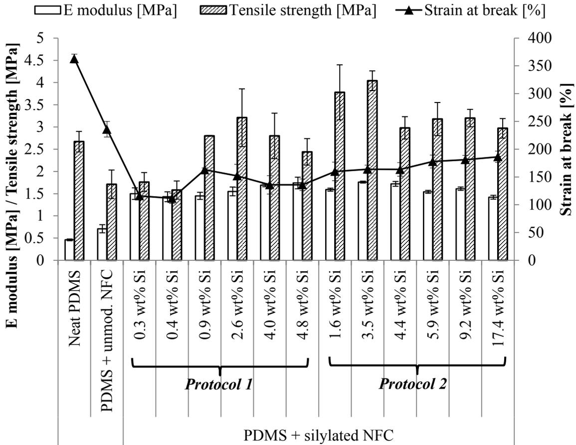
**Figure 46: Elastic modulus (E), tensile strength ( $\sigma$ ) and strain of break ( $\epsilon$ ) of PDMS composites containing 1 % NFC treated at different  $[MTMS]_i$  according to *Protocol 1* or *Protocol 2*.**
