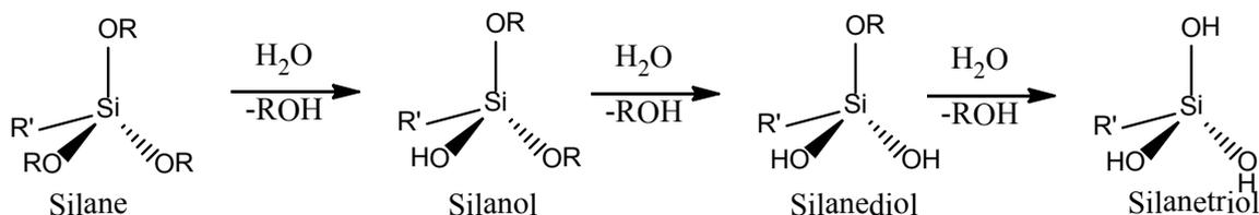
**Scheme 16: Step-wise hydrolysis of trialkoxysilanes.**<sup>166</sup>
