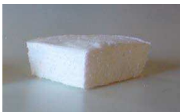
Figure 11: Image of NFC foam prepared by the freeze-drying method. 104
