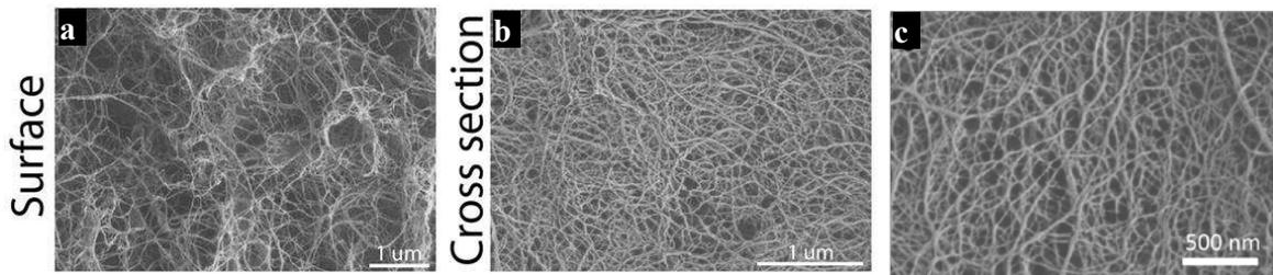
**Figure 13: SEM micrographs of NFC aerogels prepared by t-butanol freeze drying (a and b)<sup>104</sup> and supercritical CO<sub>2</sub> drying (c)<sup>113</sup>**
