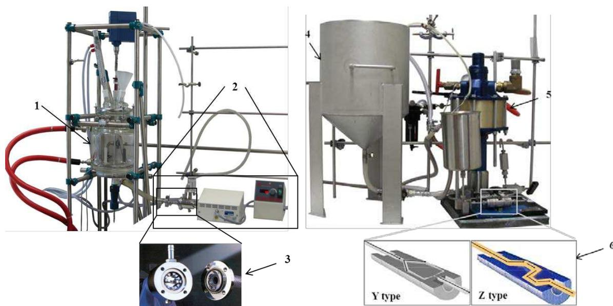
**Figure 65: Demonstration of NFC production process: 1. Swelling of cellulose suspension in 10L reactor. 2. Pretreatment with homogenizer (inline Ultra-Turrax system). 3. Inside Ultra-Turrax system. 4. After pretreatment, cellulose suspension was**
