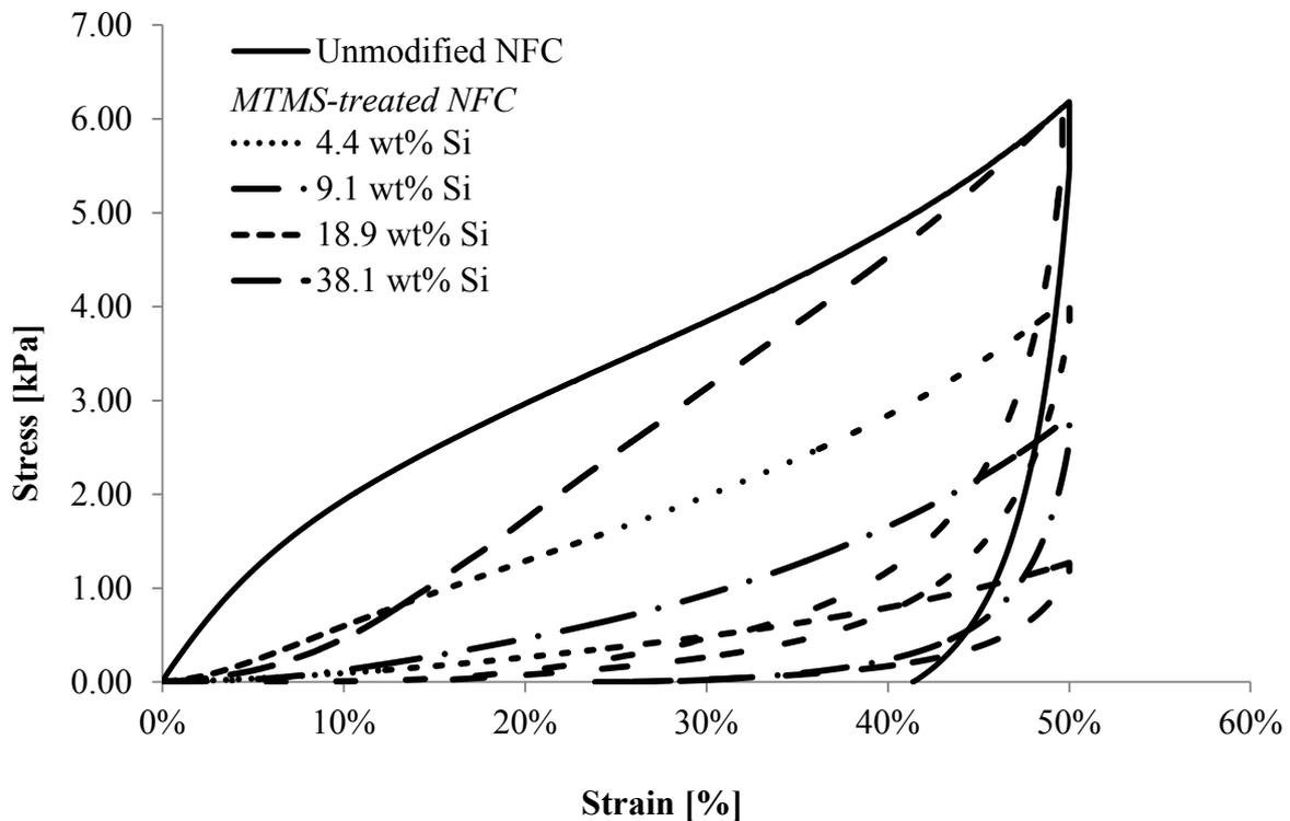
**Figure 56: Compressive stress-strain curves of unmodified NFC foam and silylated NFC foams, prepared at different [MTMS]<sub>i</sub> according to Protocol 2'.**
