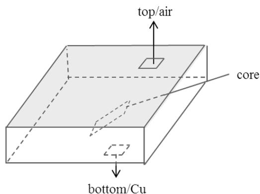
**Scheme 21: Sketch of a foam prepared according to *Protocol 2*'. "Top" refers to the surface in contact with air during freezing; "bottom" refers to the surface which was in contact with the copper mold.**
