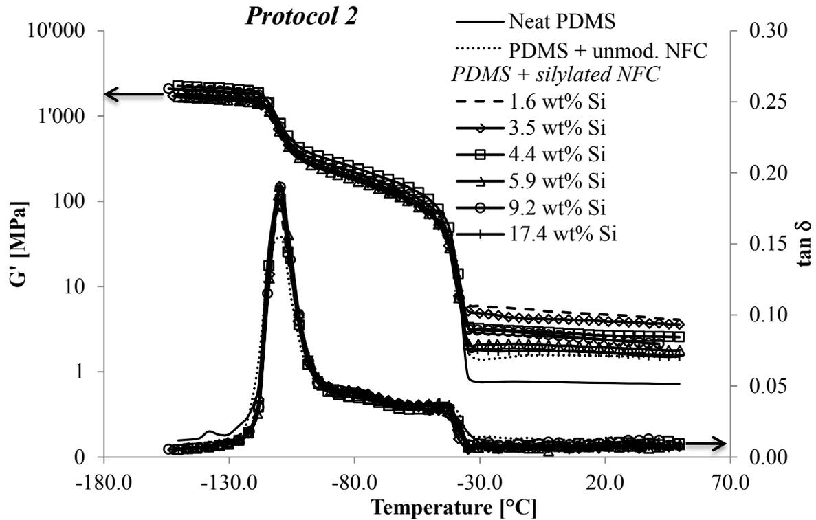
**Figure 44: Temperature-dependant shear modulus and damping factor ( $\tan\delta$ ) of PDMS composites containing 1 % NFC treated at different [MTMS]<sub>i</sub> (*Protocol 2*).**
