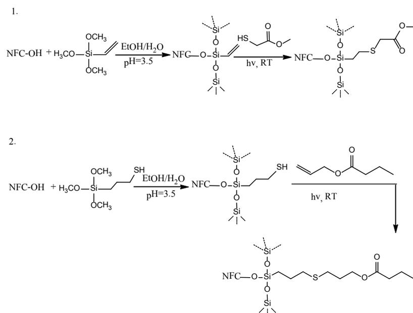
**Scheme 14: Functionalization of NFC by silylation and subsequent thiol-ene coupling.<sup>147</sup>**
