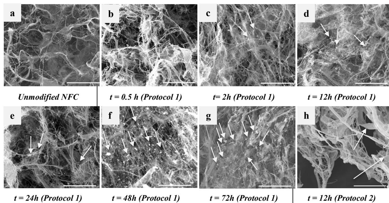
**Figure 26: SEM micrographs of unmodified NFC (a) and NFC treated with MTMS according to *Protocol 1* (b-g) or *Protocol 2* (h) (Scale bar is 10  $\mu\text{m}$ ). Results with various reaction times are presented.**
