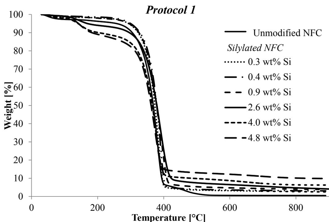
**Figure 41: Thermograms of unmodified NFC and NFC treated at different [MTMS]<sub>i</sub> with *Protocol 1*.**
