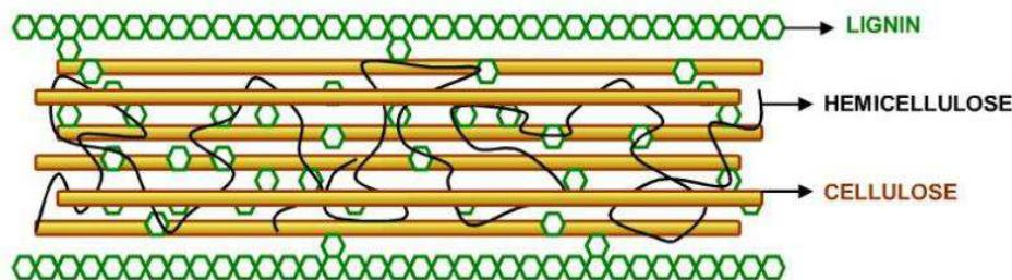
**Figure 5: Representation of lignocellulose structure<sup>31</sup>**
