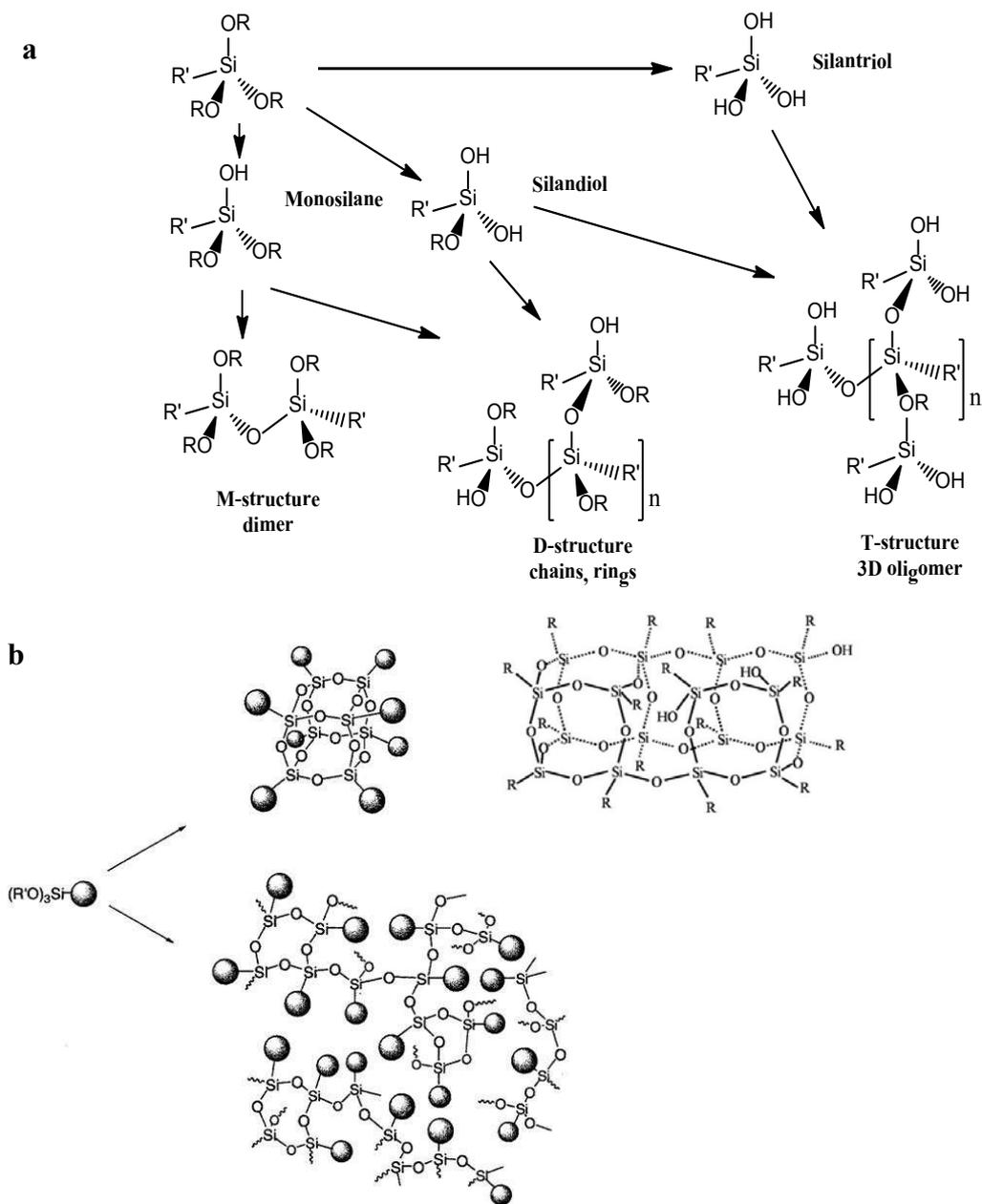
**Scheme 18: (a) Oligomers formed during hydrolysis and condensation.<sup>167</sup> (b) Examples of oligomer structures: cage-like structures (upper)<sup>168, 169</sup> and various amorphous species (lower)<sup>169</sup>**
