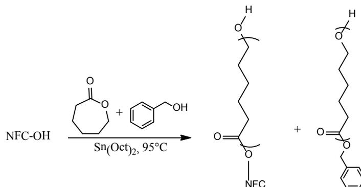
**Scheme 15: Grafting of PCL on NFC by ring-opening polymerization.**<sup>153</sup>
