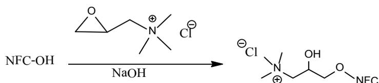
**Scheme 7: Etherification of NFC with glycidyltrimethylammonium chloride**
