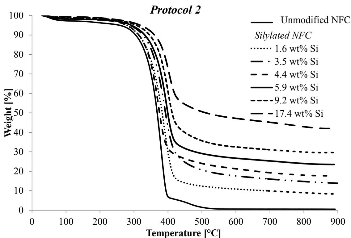
**Figure 42: Thermograms of unmodified NFC and NFC treated at different [MTMS]<sub>i</sub> with *Protocol 2*.**
