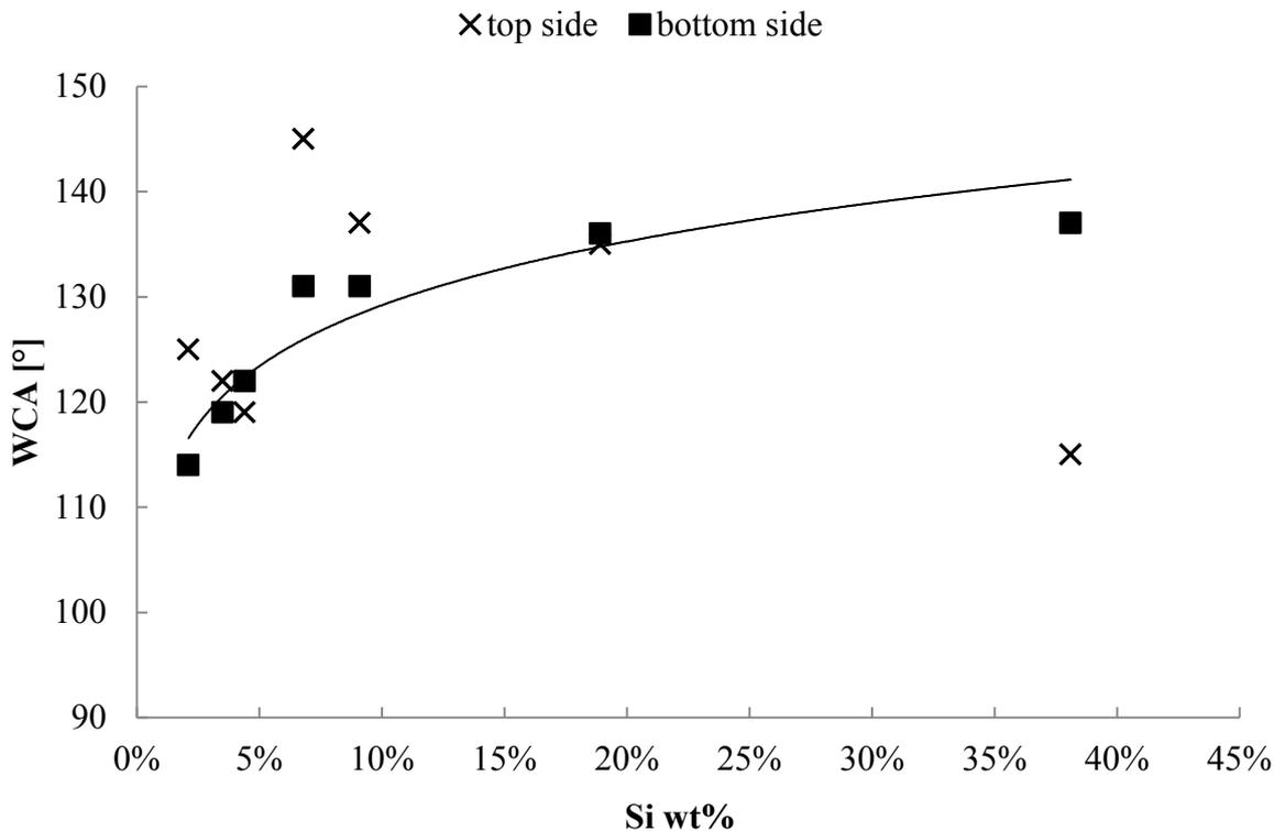
**Figure 58: Water contact angle values (WCA) measured at the surface of NFC foams treated at different [MTMS]<sub>i</sub> according to *Protocol 2*'.**
