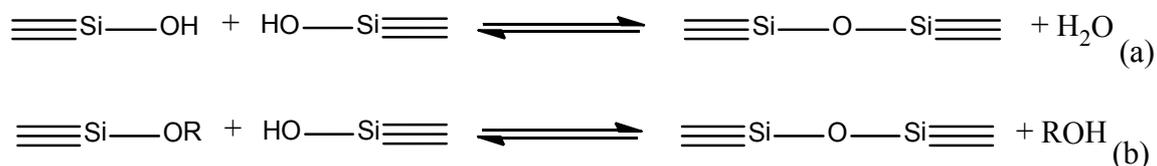
**Scheme 17: Formation of siloxane linkages by condensation reactions**<sup>160</sup>
