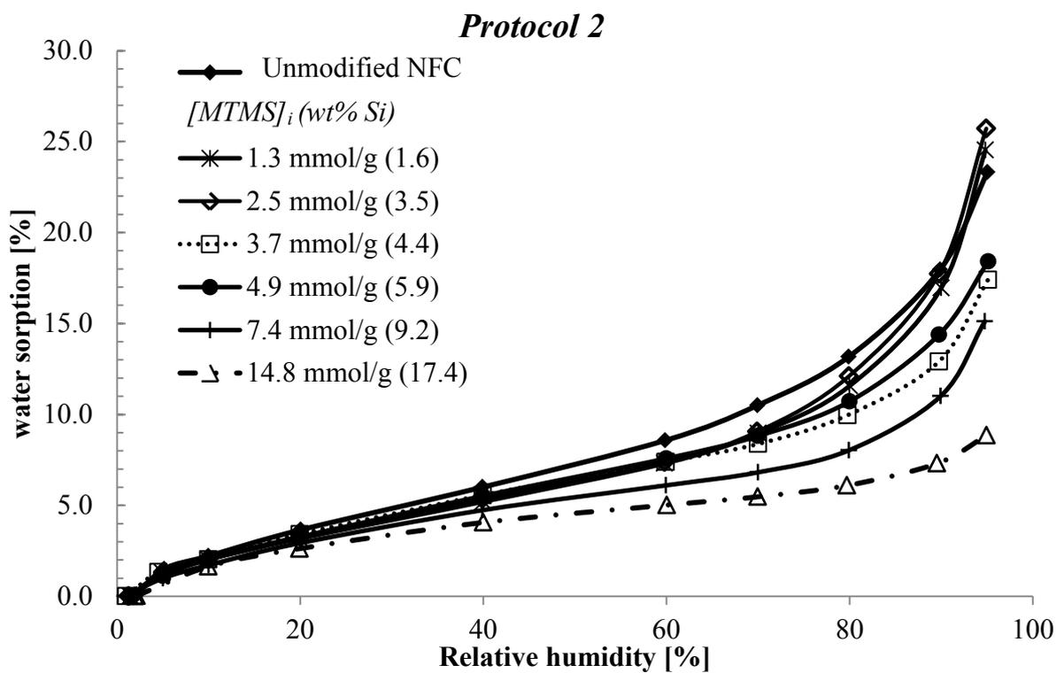
**Figure 40: Water sorption isotherms of unmodified NFC and NFC treated at different  $[MTMS]_i$  according to *Protocol 2* ( $T = 23\text{ }^\circ\text{C}$ ).**
