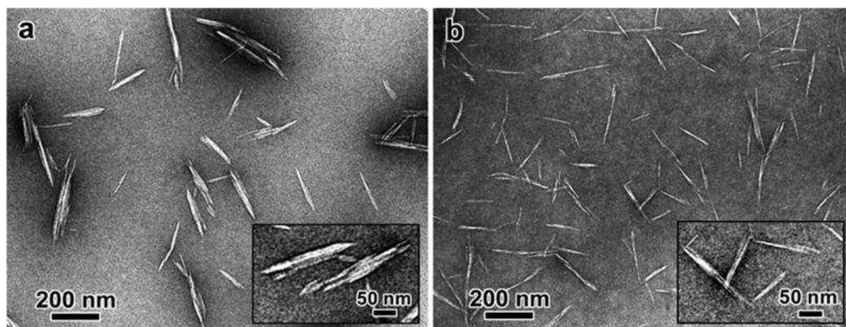
**Figure 7: TEM micrographs of CNC obtained by sulfuric acid hydrolysis of cotton (a), and MCC (b).<sup>40</sup>**
