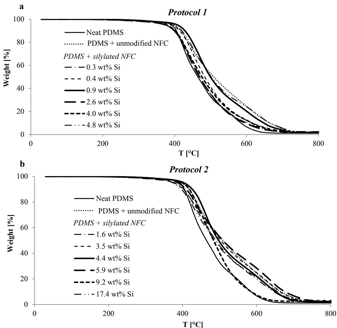
**Figure 47: Thermograms of PDMS composites containing 1 wt % unmodified or MTMS-treated NFC (a: *Protocol 1* and b: *Protocol 2*).**
