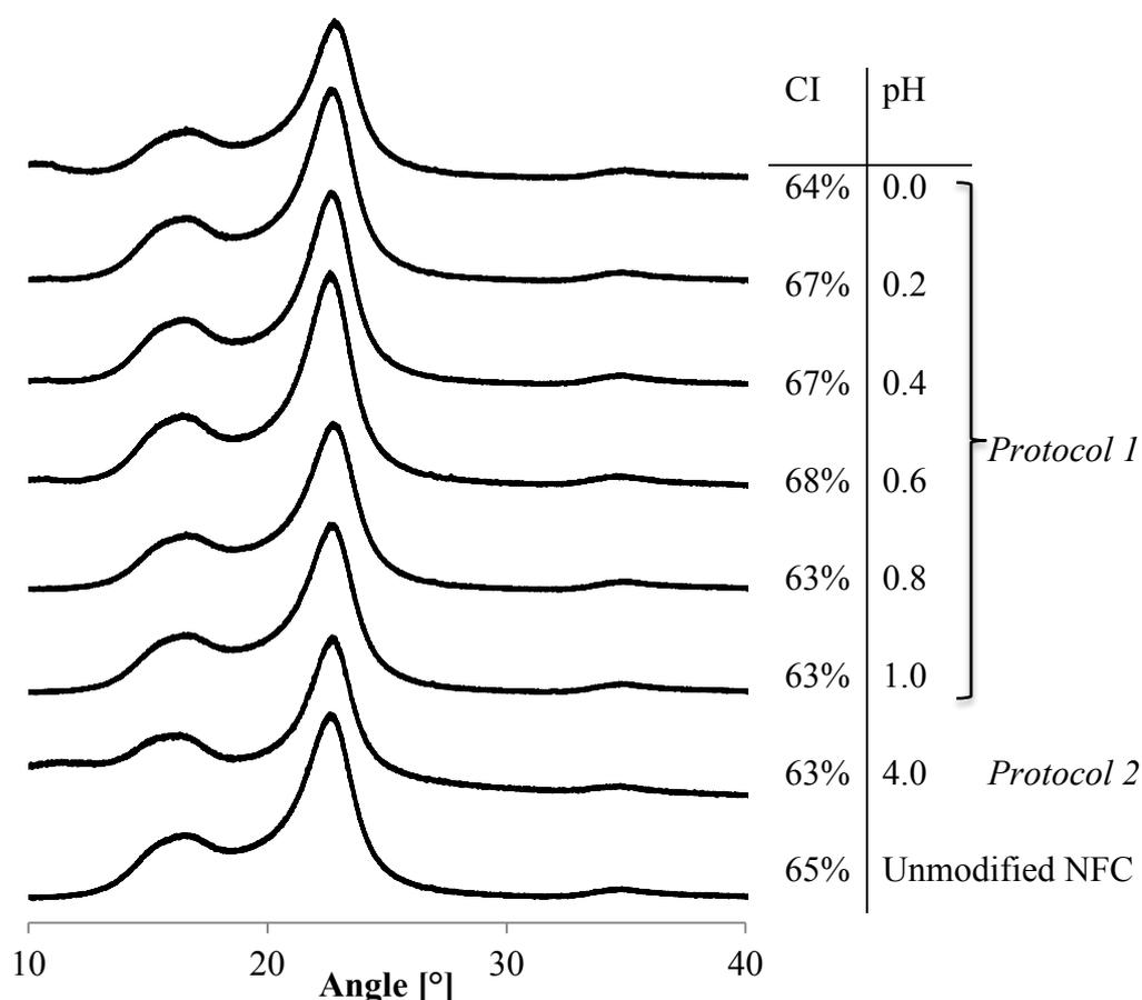
**Figure 37: XRD profiles of unmodified NFC and NFC treated with MTMS at different pH with *Protocol 1* (pH = 0 - 1) or *Protocol 2* (pH = 4).**
