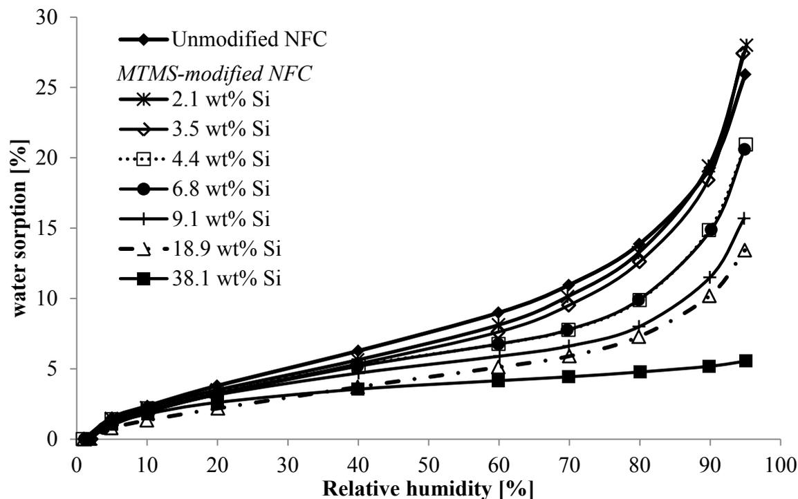
**Figure 59: Water sorption isotherm of unmodified NFC foam and NFC foams prepared at different [MTMS]<sub>i</sub> according to Protocol 2' (T = 23 °C).**
