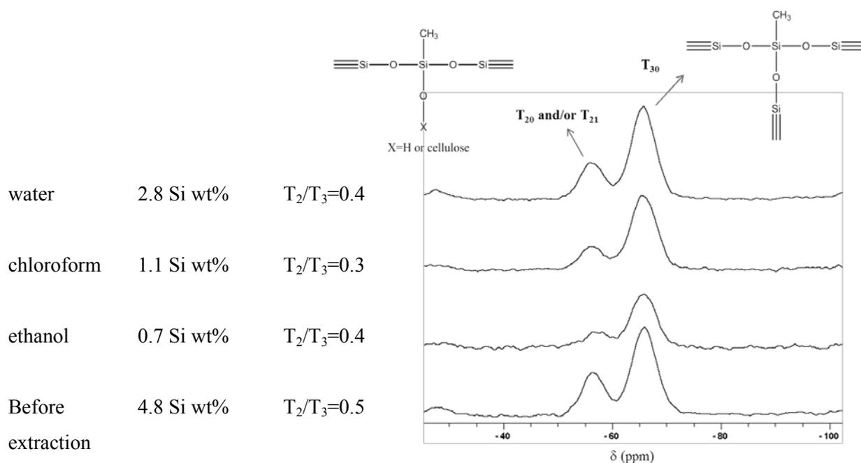
**Figure 35:**  $^{29}\text{Si}$  CP-MAS NMR of NFC treated by 14.8 mmol MTMS/g<sub>NFC</sub> (*Protocol 1*), before and after extraction with water, chloroform and ethanol.
