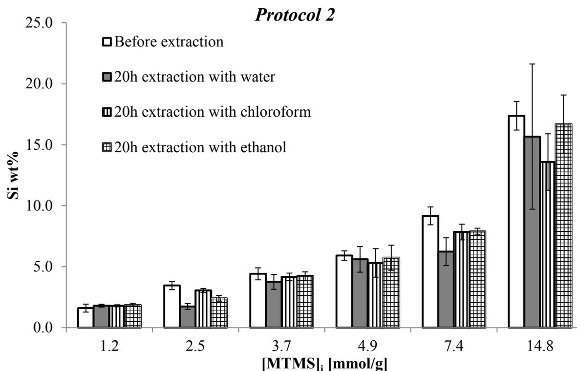
**Figure 36: Evolution of the Si content in MTMS-treated NFC prepared at different [MTMS]<sub>i</sub> (*Protocol 2*), before and after extraction with water, chloroform and ethanol.**
