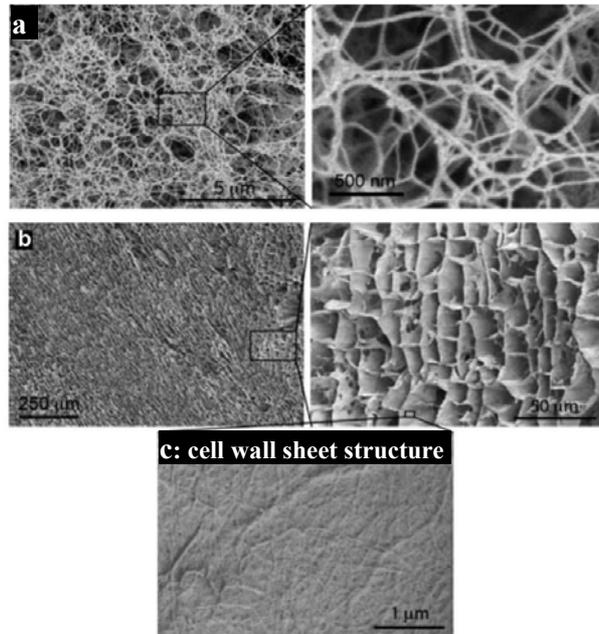
**Figure 12: SEM images of NFC foams obtained by freeze-drying: a) Fast freezing (bottom layer); b-c) Slow freezing (layer > 3 mm).<sup>111</sup>**
