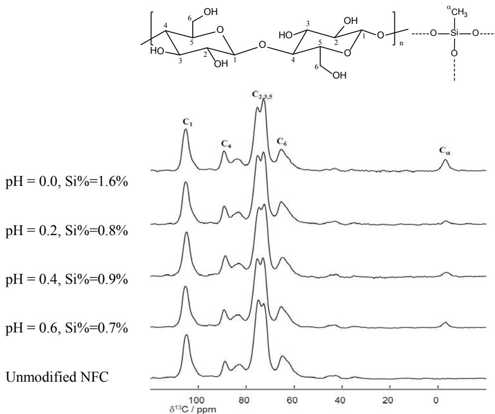
**Figure 17:  $^{13}\text{C}$  CP-MAS NMR spectra of unmodified and MTMS-modified NFC prepared at different pH**
