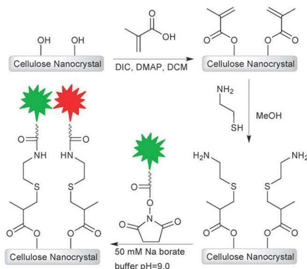
**Scheme 13: Fluorescent labelling of cellulose nanocrystals by thiol-ene reaction<sup>152</sup>**
