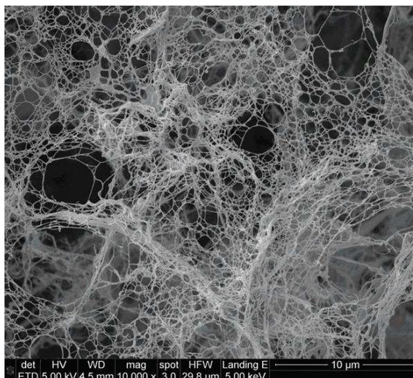
**Figure 8: SEM micrograph of NFC, mechanically isolated from oat straw cellulose powder<sup>12</sup>**
