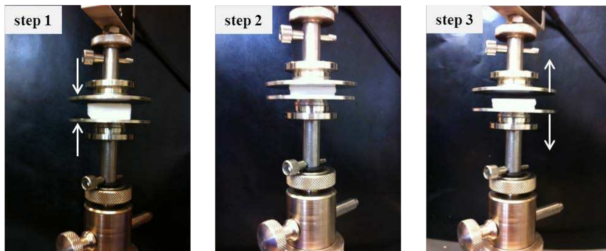
Figure 67: Experimental set-up used for compression tests. The testing plates movement is symbolized by arrows.
