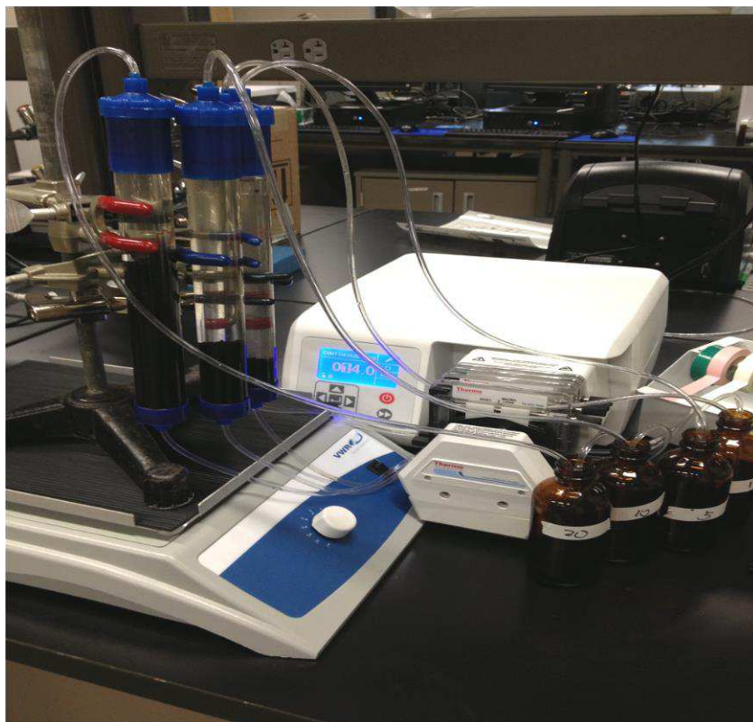
Fig. 8.2. Saturated filter columns with varying volumes of sampled BAC media.
