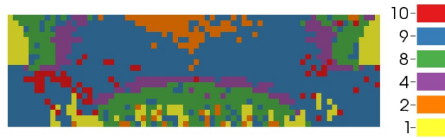
Figure 7.65: Solution type of local minimisation of F_{Hill}^{Lam} , algorithm a priori version 2, rectangular plate: different tension/compression strength.
