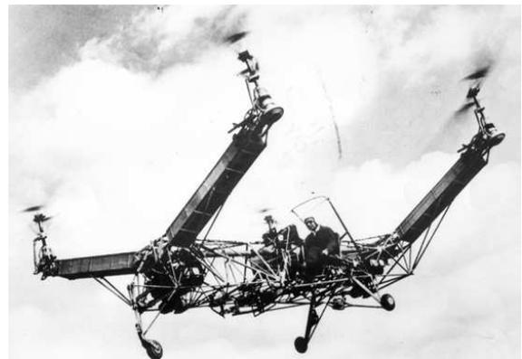
Figure 1.5: Convertawings Model A. (The source: [www.aviastar.org](http://www.aviastar.org).)
