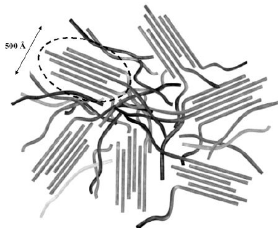
Figure 2.5: Schematic representation of an entangled network of elongated rodlike aggregates in Nafion. Long-range heterogeneities arising from bundles of locally ordered aggregates. Figure from reference [Rubatat 2004]
