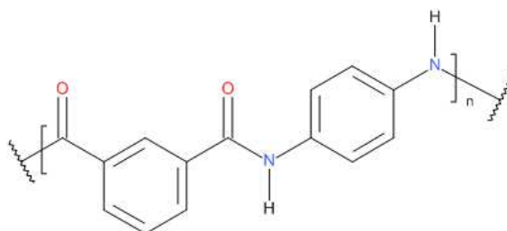
Figure 2.4: Poly(phenylene isophthalamide), also named Nomex ®
