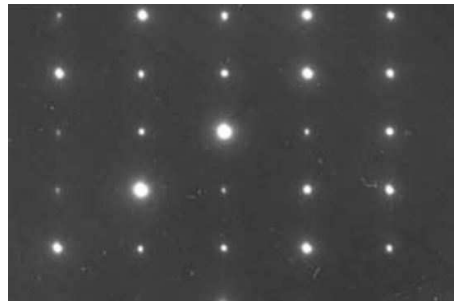
FIGURE 3.3 – Cliché de diffraction d'un cristal bcc (001) [1]
