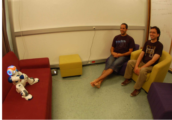
Figure 6.1: A typical scenario in which a companion humanoid robot (NAO) performs audio-visual fusion in an attempt to detect the auditory status of each one of the speakers in the room. The system described in this chapter processes the raw data gathered with the robot’s camera and microphone pairs. The system output is a speaking probability of each one of the actors together with the 3D location of the actors’ faces.
