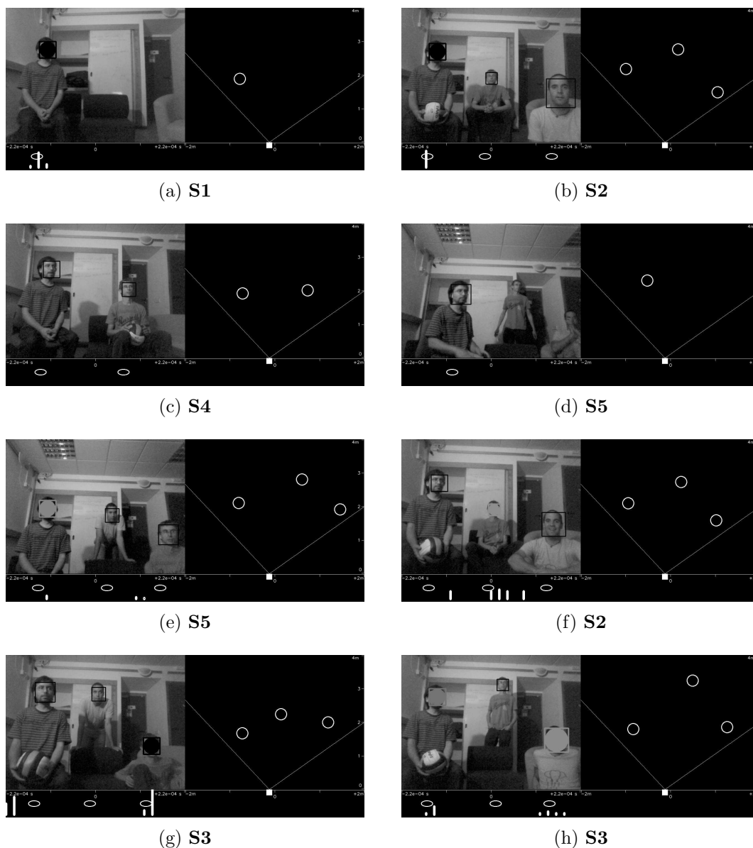
Figure 6.4: Snapshots of the visualization tool. Frames are selected among the five scenarios such as to show both the method's strengths and weaknesses. (a) Good results on S1 . (b) Good results on S2 , three people. (c) The ITD extractor does not work correctly, thus missing the speaker. (d) Misses of the face detection module. (e) The audio-visual fusion fails to set a high probability to the current speaker. (f,g) The audio-visual fusion model is able to handle reverberations. (h) The reverberations are too close to the mapped head, leading to a wrong decision.
