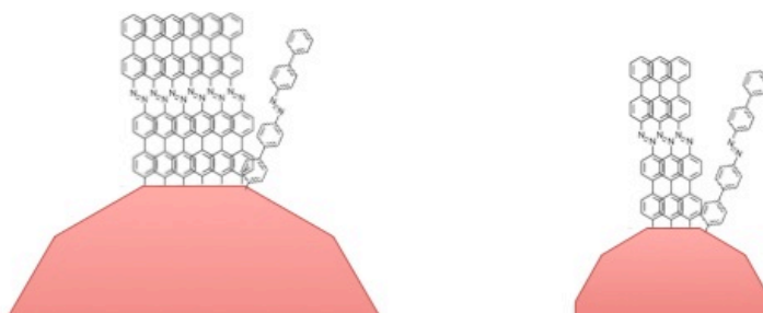
Figure 4.2.1 Sketch of the shape of the nanoparticles employed in kinetic studies. At the left 15 nm gold nanoparticles and at the right 3 nm gold nanoparticles.
