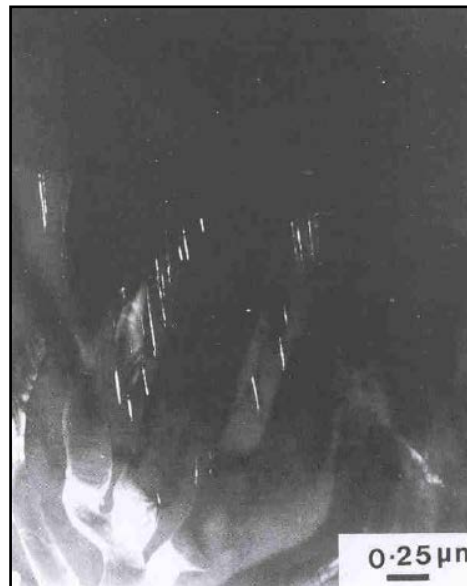
Figure 2-11 The observed fibrous carbides in pearlitic ferrite, a dark-field image [5]
