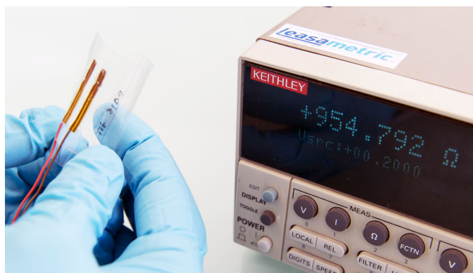
Figure 2.8: In-situ measurement of the electrical conductivity during mechanically folding an undoped CVD graphene layer transferred onto polyethylene film. Prospect of using graphene for flexible electrodes is great, as ITO is brittle and cannot be folded.
