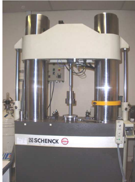
FIGURE 1.9 – Machine servo-hydraulique SCHENCK VHF7 [152].
