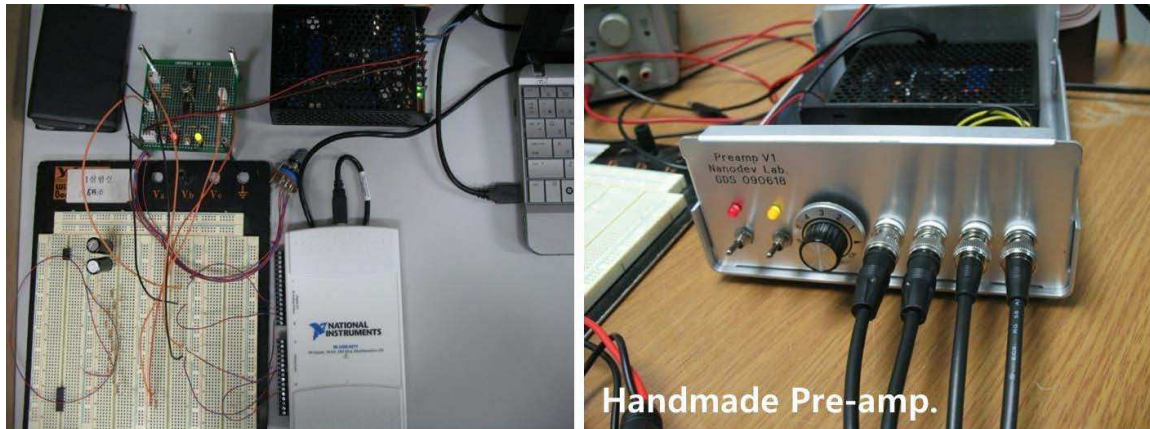
Figure 10. Electrometer systems with NI-DAQ and handmade Pre-amplifier.
