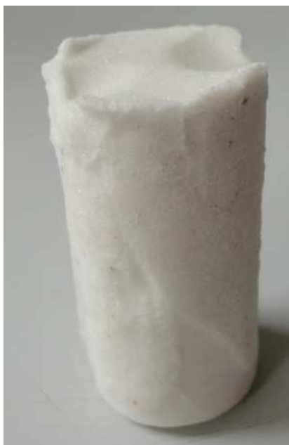
Figure 12.4: Sintered glass core obtained with a plaster mould.
