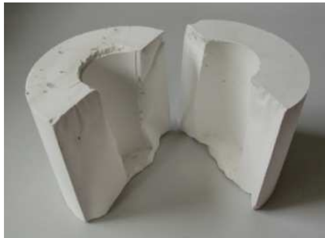
Figure 12.3: Plaster mould used for glass sintering.
