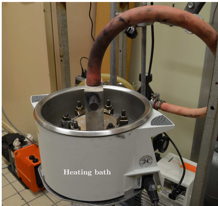
FIGURE 3.6: Creating vacuum inside the container. The container is placed into a heating bath to favor the powder drying.
