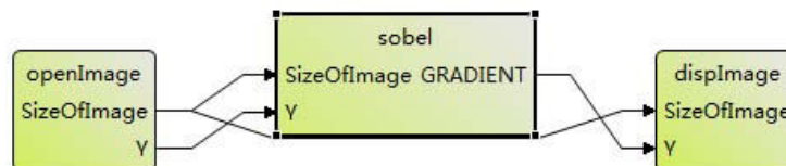
Figure 2.6: Sobel Filter XML Dataflow Format
