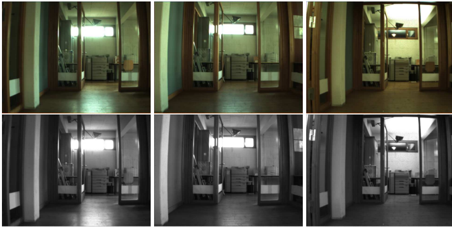
Figure 4.2: First row: color images acquired under three different illumination conditions (sunny, cloudy, and night) respectively. Second row: the corresponding gray-scale images. It is obvious that the illumination variations reduced in the case of gray images.
