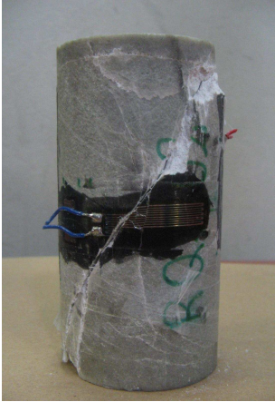
Figure 2.22: Failure pattern of siliceous rock under triaxial compression at 50 MPa of confinement
