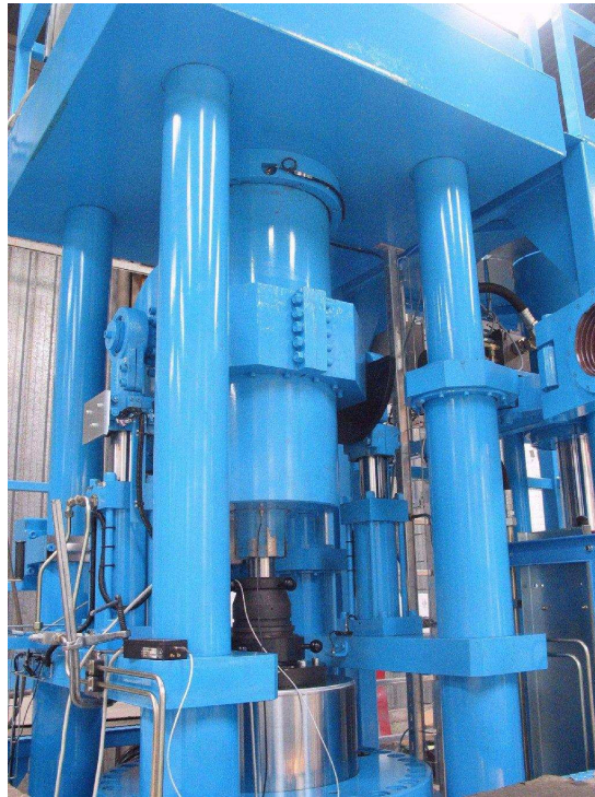
Figure 2.1: Overview of the triaxial press GIGA
