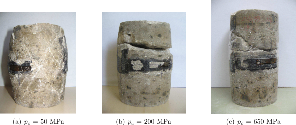
Figure 2.33: Failure patterns in LC specimen under different triaxial compression tests
