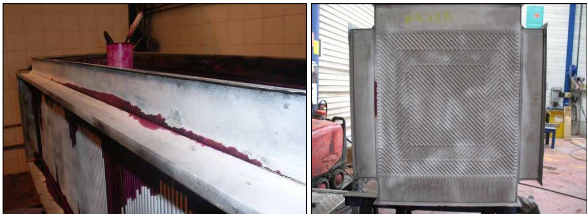
Figure I.14 - Failure in two welded zones
